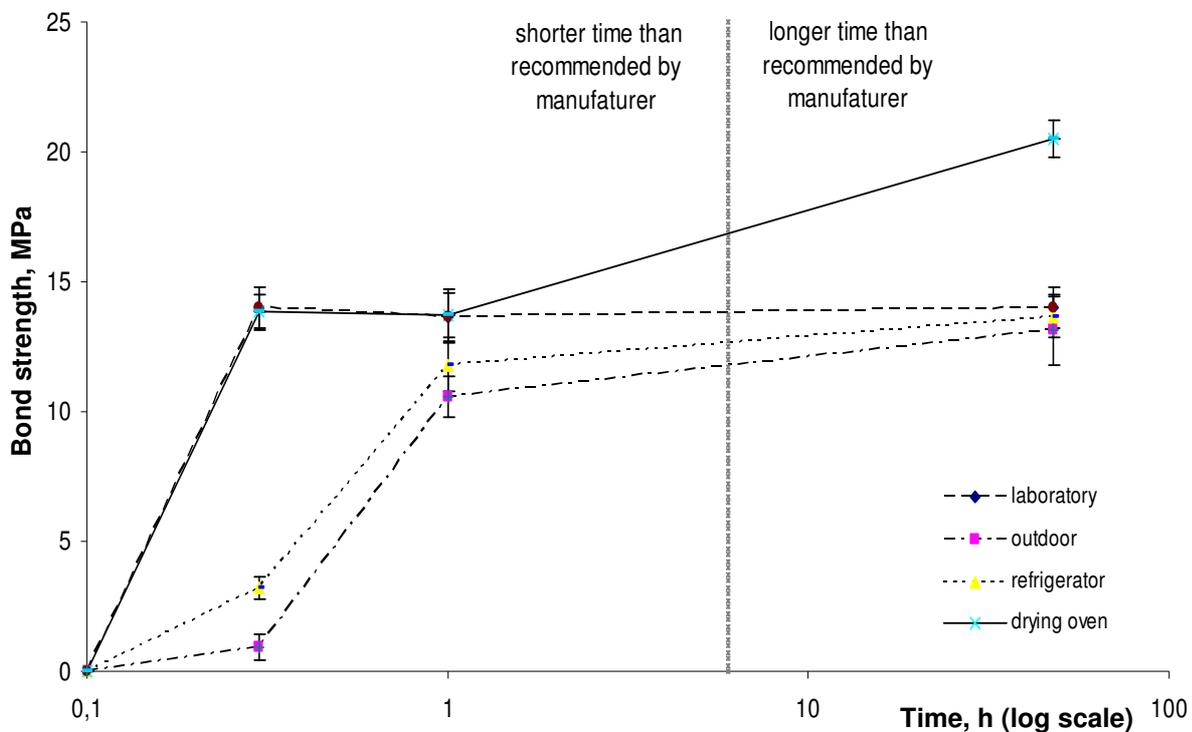
Fig. 2. Influence of curing time on bond strength
