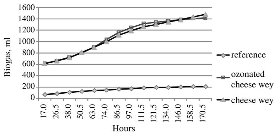
Fig. 3. Cumulative amount of biogas in Experiment 2
