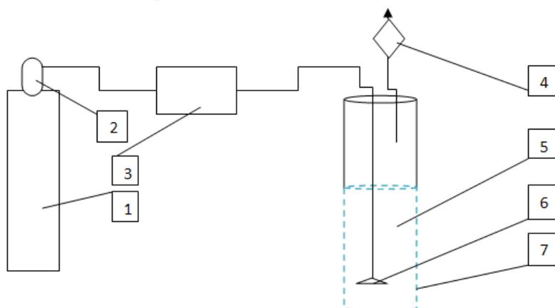
Fig. 1. **Scheme of ozonation equipment:** 1 – oxygen cylinder; 2 – pressure regulator; 3 – ozone generator; 4 – ozone destructor; 5 – cheese whey; 6 – diffuser; 7 – glass cylinder
