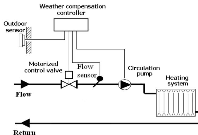
Fig. 1. Principal scheme of heating substation
