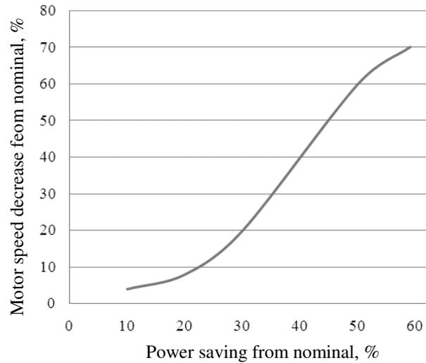
Fig. 4. Electrical power saving by pumps motor speed decrease rate from nominal ones
