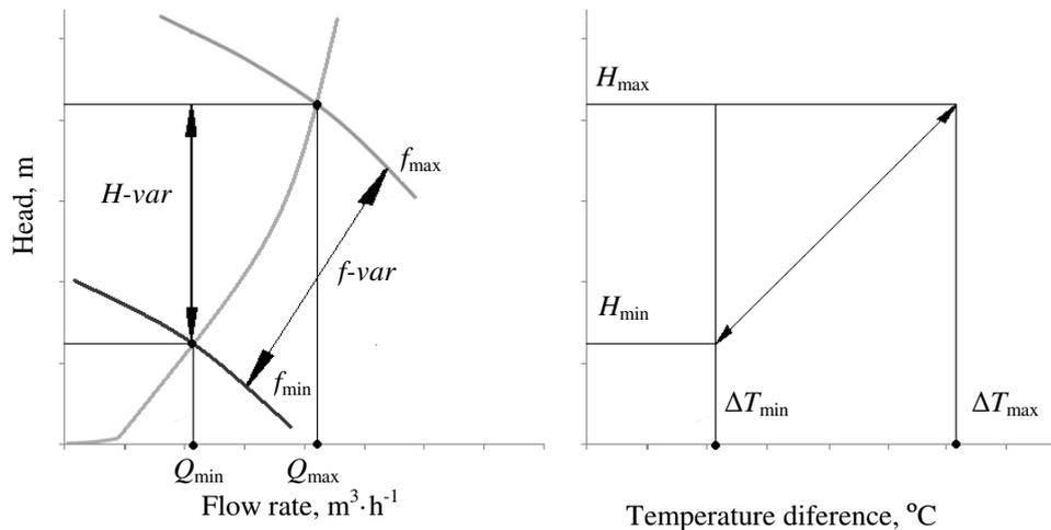
Fig. 6. Pump control by temperature difference  $\Delta T$
