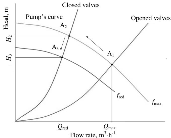
Fig. 5. Head reduction at frequency control by flow rate compared to the one at throttling
