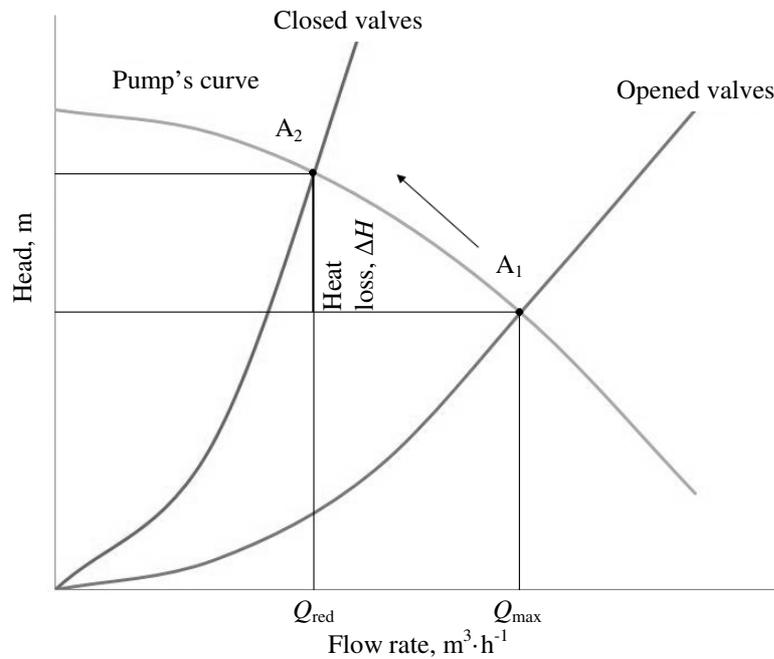
Fig. 2. Pump and heating system curves at throttling
