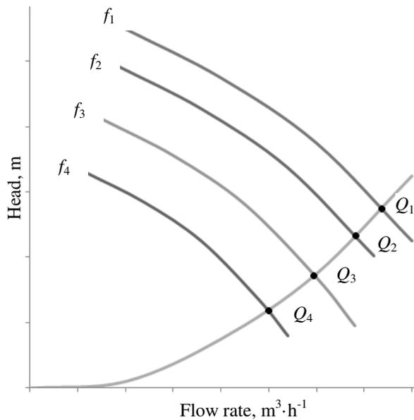
Fig. 3. Flow control by motors frequency change
