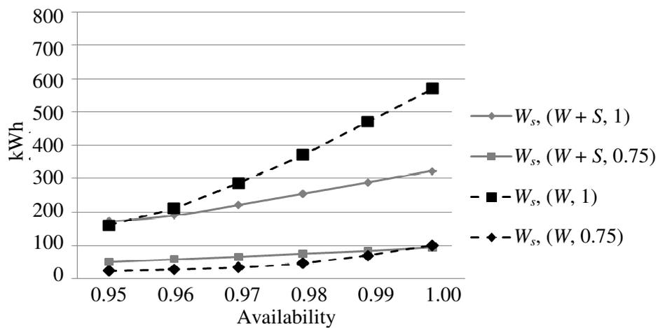
Fig. 3. Necessary accumulation availability  $W_s$  by different consumption factors  $\beta = 0.75$  and  $\beta = 1.0$  in case of two solutions: only wind (W) and wind+solar (W+S)
