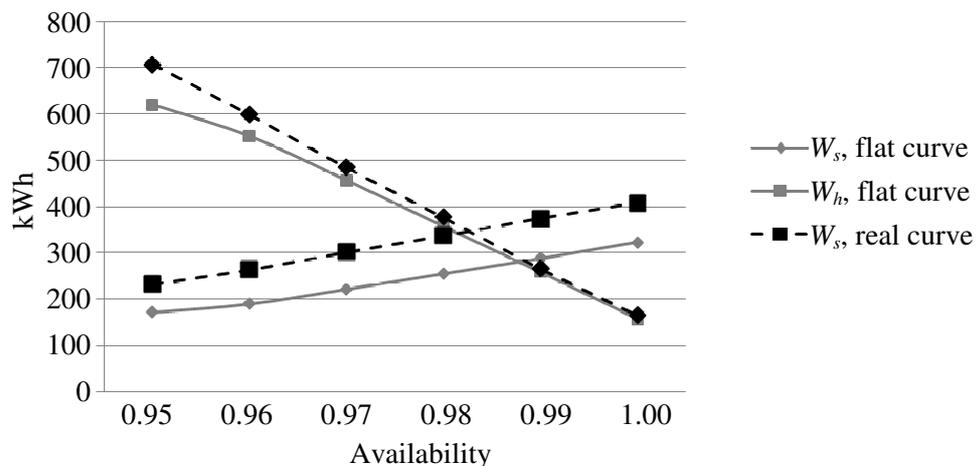
Fig. 2. Necessary storage capacity and heat energy according to availability, when  $\beta = 1$  wind+solar solution by flat and real consumption curves
