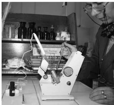
Fig. 3. Determination of refractive index
