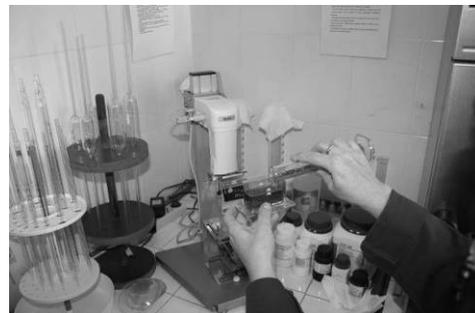
Fig. 2. Determination of oil viscosity
