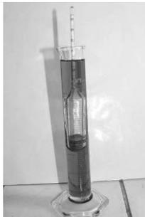
Fig. 1. Determination of oil density
