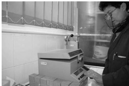
Fig. 4. Determination of calorific power
