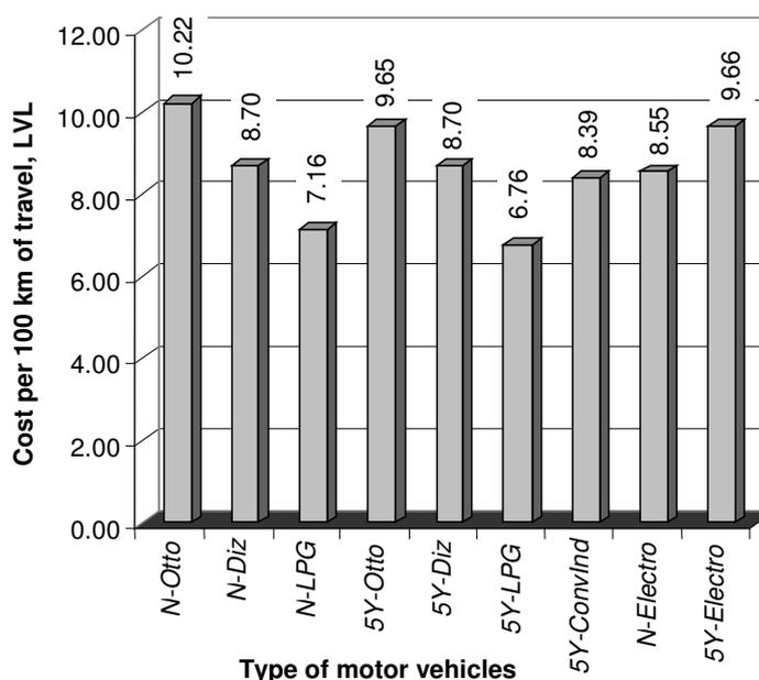
Fig. 1. Total relative costs for various types of motor vehicles, LVL·(100 km)<sup>-1</sup>
