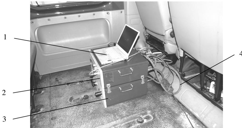
Fig. 1. AVL KMA Mobile fitted to automobile: 1 – computer for data collecting; 2 – measuring module; 3 – conditioning module; 4 – fuel supply hoses
