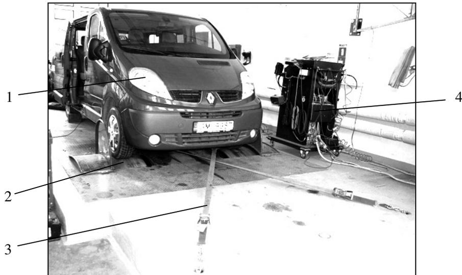
Fig. 3. Renault Traffic on chassis dynamometer:
