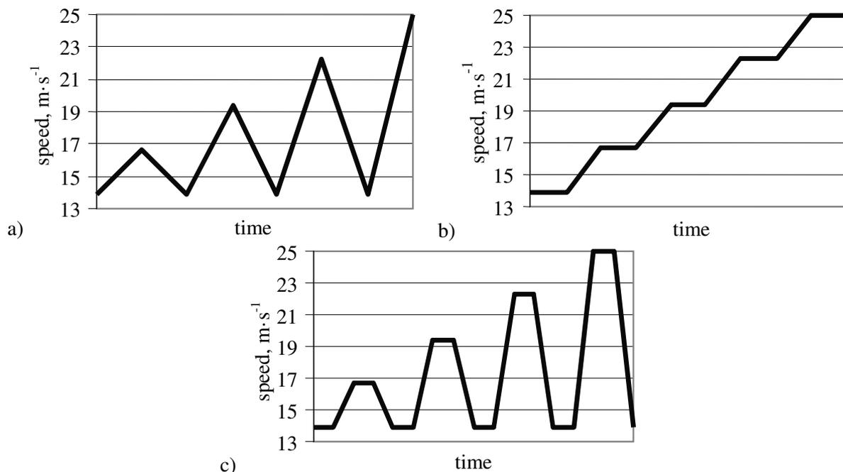
Fig. 4. Driving cycles: a – pulsing; b – gradual; c – impulse
