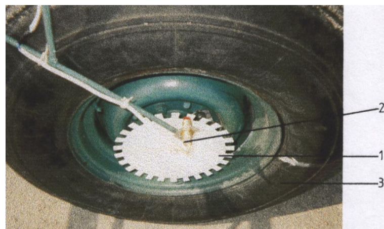
Fig. 3. Induction disc and proximity transducer location: 1 – induction disc; 2 – proximity transducer; 3 – transport wheel
