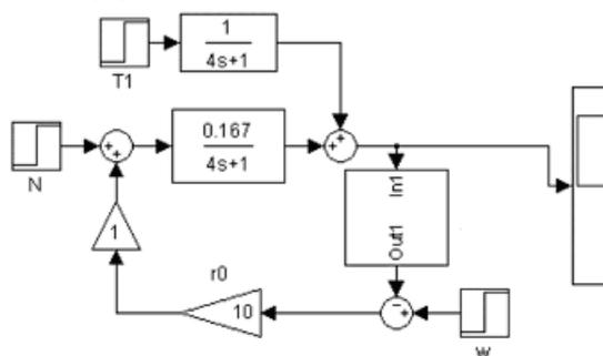
**Fig. 8. Flowchart of the control circuit**
