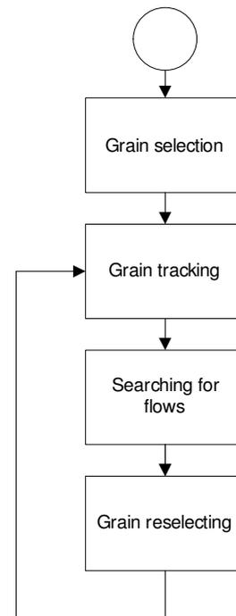
Fig. 2. Algorithm for granular flow recognition
