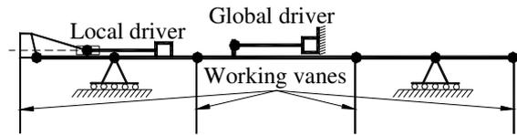
Fig. 8. A manure scraper with local driver driven manipulator
