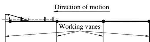
Fig. 2. **Novel manure scraper for manure press removal**
