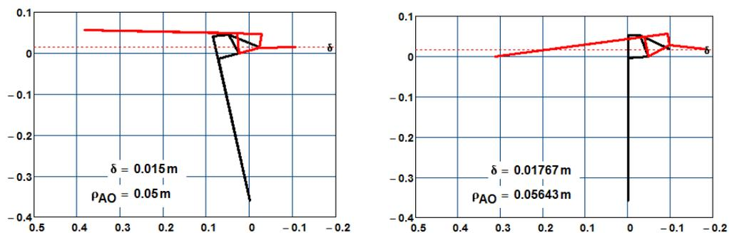
**Fig. 4. Positions of virtual manipulator before (left) and after optimization (right)**
