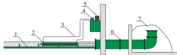
Fig. 1. **Principal scheme of press manure removal:** 1 – one-sided scraper; 2 – hydraulic cylinder; 3 – oil pipe; 4 – valve; 5 – electric engine; 6 – manure pipe; 7 – heap of muck
