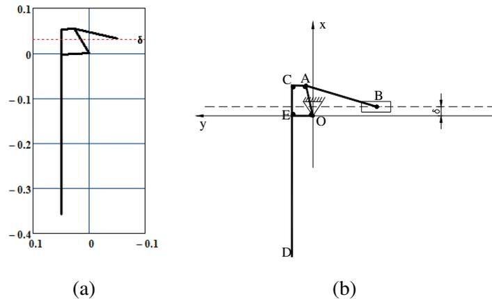
**Fig. 3. Virtual model (a) and computational scheme (b) of the manipulator in Fig. 2:**
