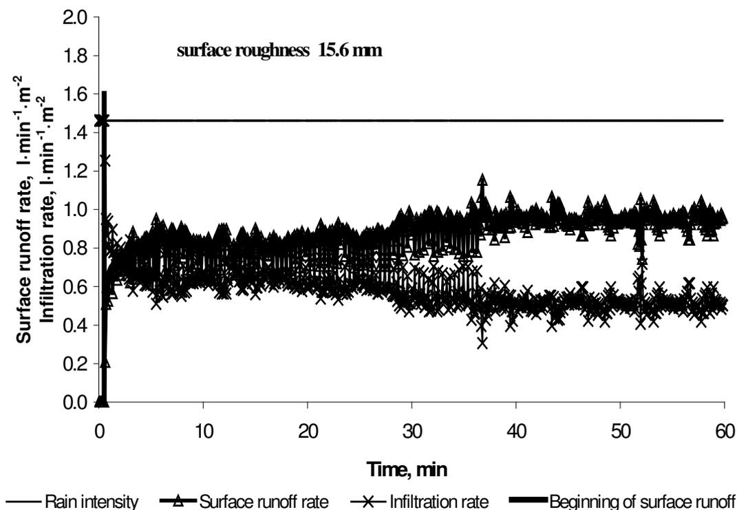
Fig. 3. Process of observed values during rain simulation – Variation 2
