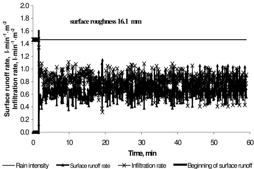
Fig. 2. Process of observed values during rain simulation – Variation 1
