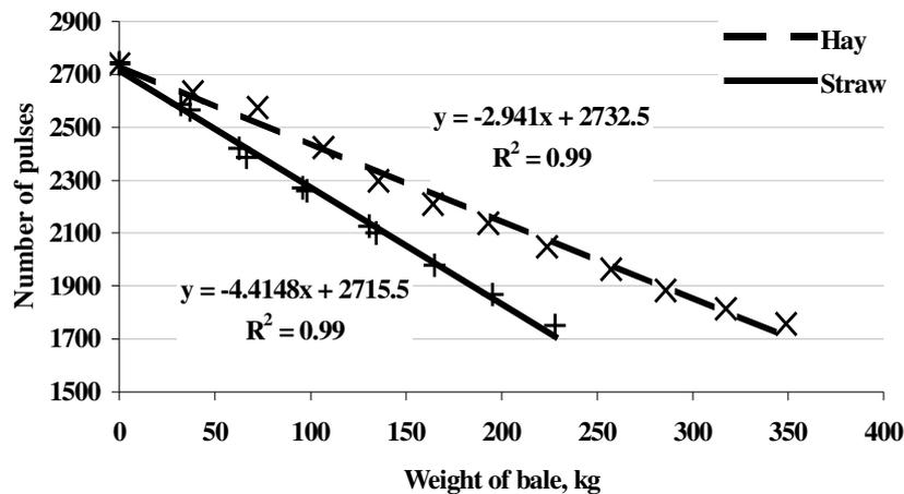
Fig. 7. Dependence of the number of pulses per bale weight for different materials
