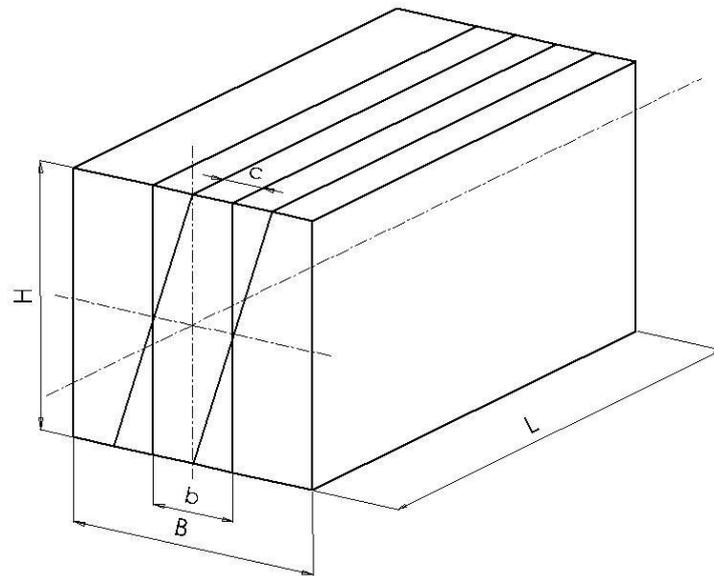
Fig. 2. A scheme of overlaying the film ribbons during wrapping of the square bale
