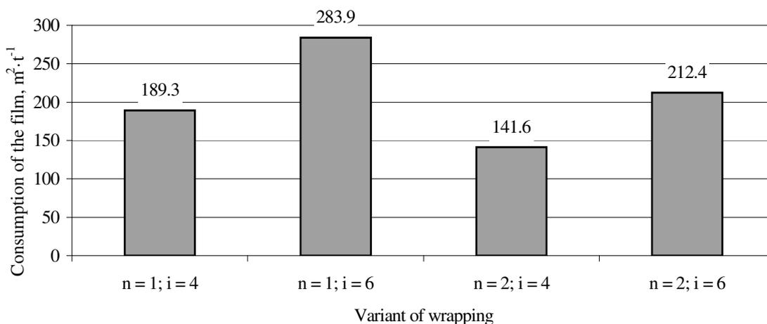
Fig. 3. Consumption of the film for wrapping bales ( $m^2 \cdot t^{-1}$  for the dry mass of the forage) with a different number of layers ( $i$ ) for the wrapping variant of a single ( $n = 1$ ) bale and of a double bale ( $n = 2$ )
