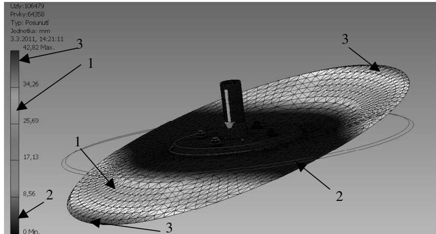
Fig. 3. Shift of individual elements during FEM analysis (80.23 Hz)
