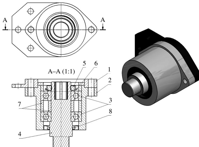
Fig. 2. Rotor of mechanical cutter:
