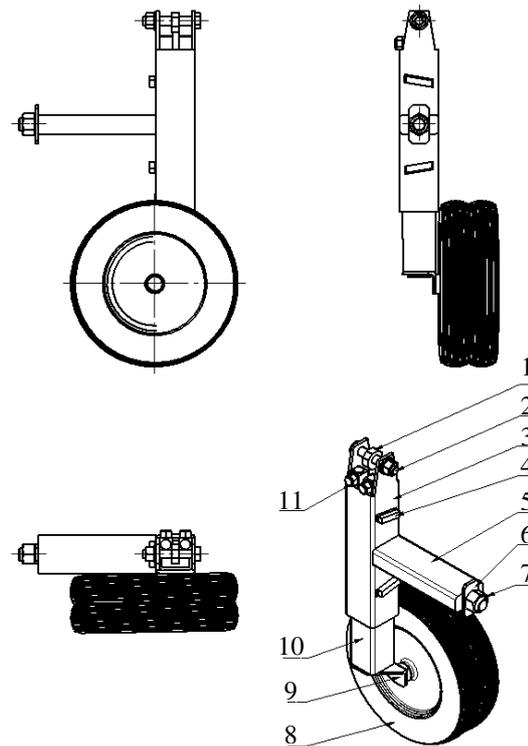
Fig. 1. Setting of cutting height (copy wheel):
