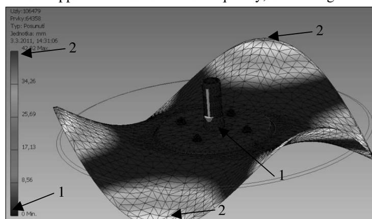
Fig. 4. Shift of individual elements during FEM analysis (146.44 Hz)
