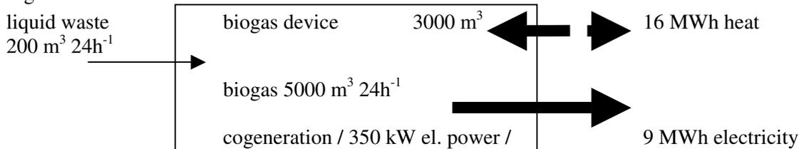
Fig. 1. 24-hour turnover of the products and energy in the procession block of liquid waste
