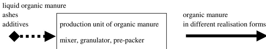
Fig. 3. Scheme of the procession block of organic manure
