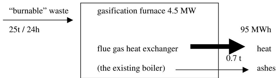
Fig. 2. 24-hour turnover of the products and energy in the procession block of burnable waste
