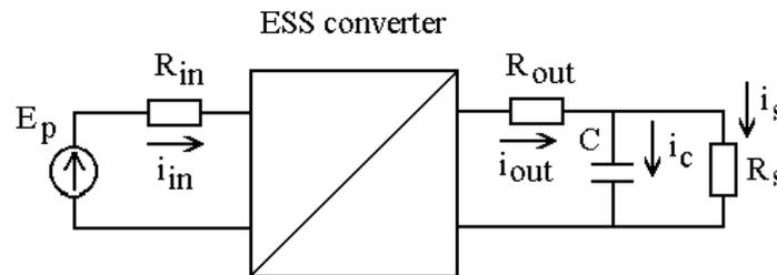
Fig. 3. Induction drive with ESS equivalent circuit
