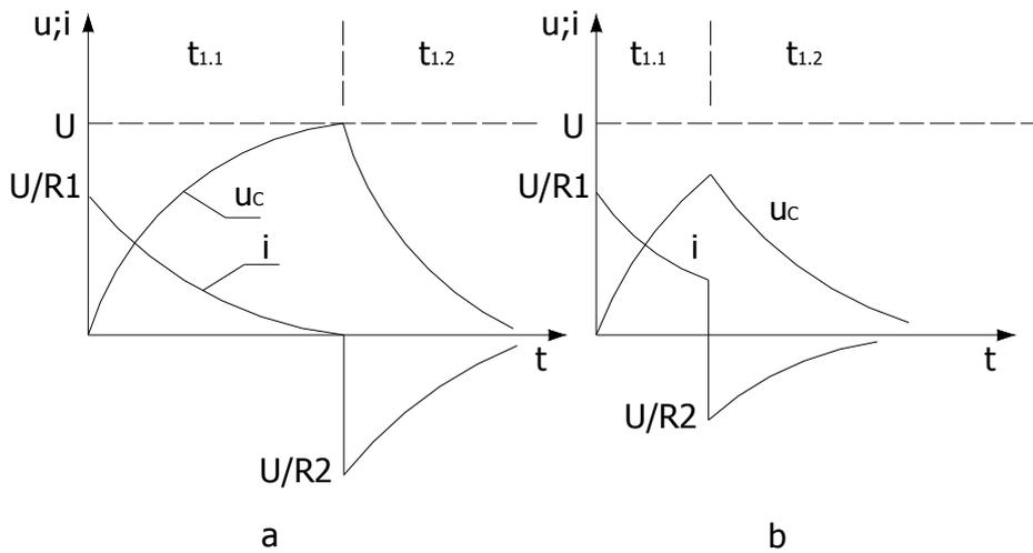
Fig. 4. Capacitor charging and discharging curves
