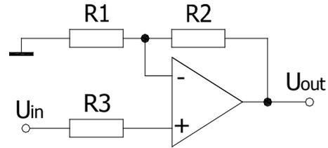
Fig 2. **Non-inverting operational amplifier circuit**
