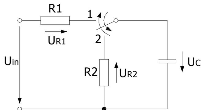
Fig. 3. Capacitor charging and discharging circuit
