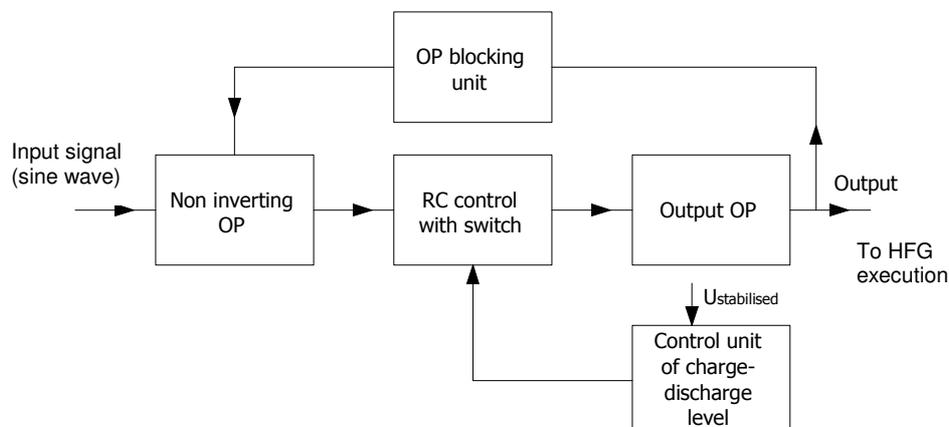
Fig. 1. Pulse density modulation circuit block diagram
