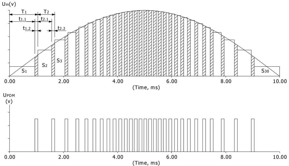
Fig. 6. Pulse density modulation circuit operation
