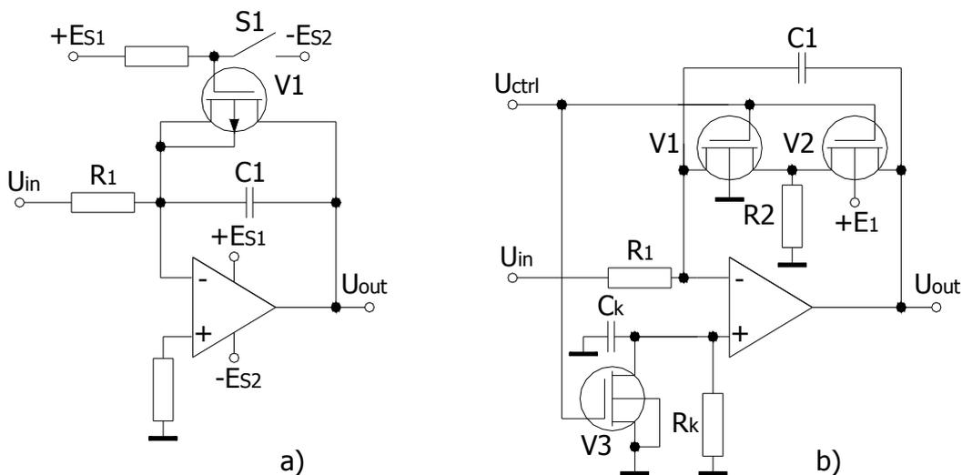
Fig. 5. Integrator reset circuits: a – with field effect transistor switch, b – with field effect transistor leakage current compensation
