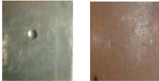
**Fig. 2. Rolled (left) and mechanically treated surfaces on samples of steel 65Mn4 after placing in a room with presence of elevated rate of hydrochloric acid steams**
