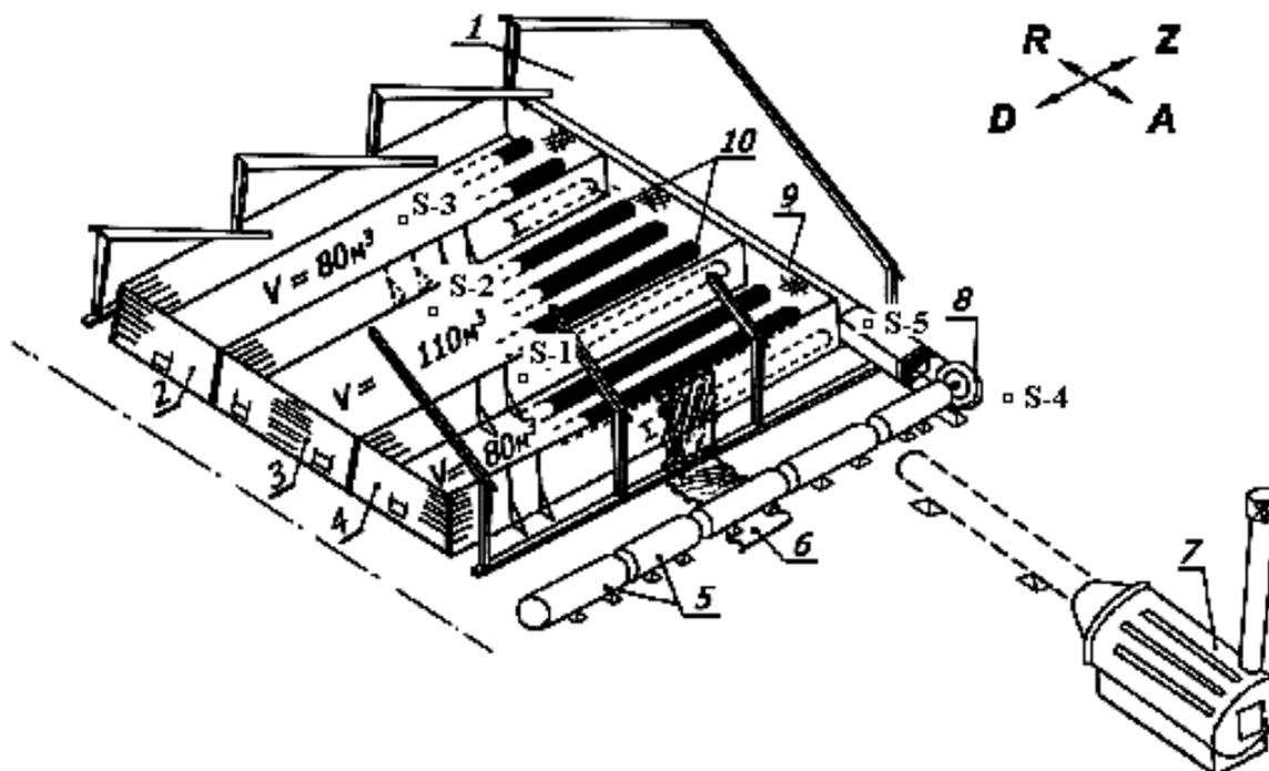
Fig. 1. A scheme of an ecological grain drier-storage plant having ventilated bins provided with sensors: 1 – the barn; 2 – 4 - ventilated grain drying-storage bins; 5 – air collectors; 6 – a solar energy absorption film; 7 – the heat generator (furnace) 40 kW; 8 – a radial fan HL 15; 9 - the main air channel; 10 – operating channels; □ S-1, □ S-2, □ S-3, □ S-4, □ S-5, □ S-6 – sensors DS1923
