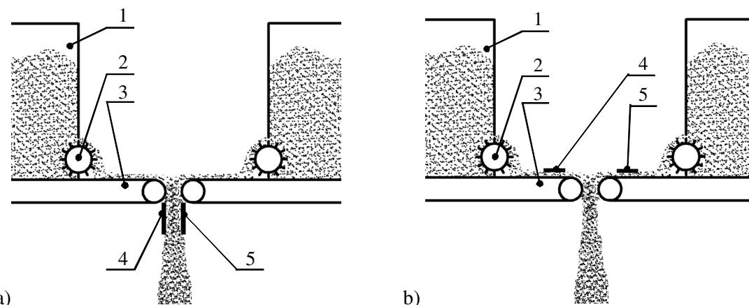
Fig. 2. In-flow mixer: 1 – container; 2 – rotor of feeder; 3 – conveyer; 4 – positive electrode; 5 – negative electrode
