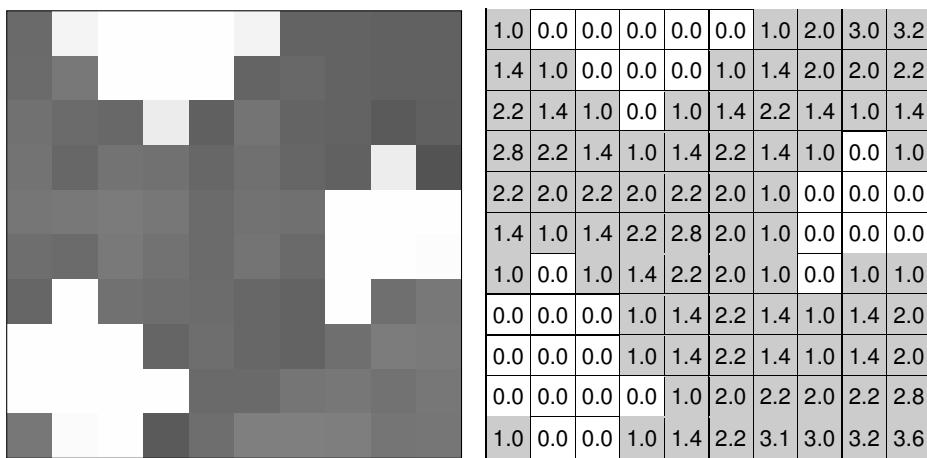
Fig. 5. Euclidian distance transformation of BW picture
