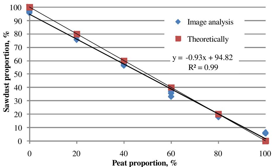
Fig. 6. Comparison data of Image analysis and theoretical data
