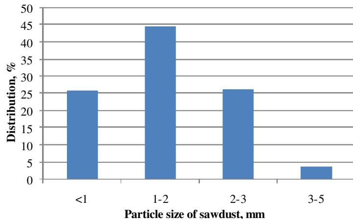
Fig.3. Distribution of particle size of sawdust
