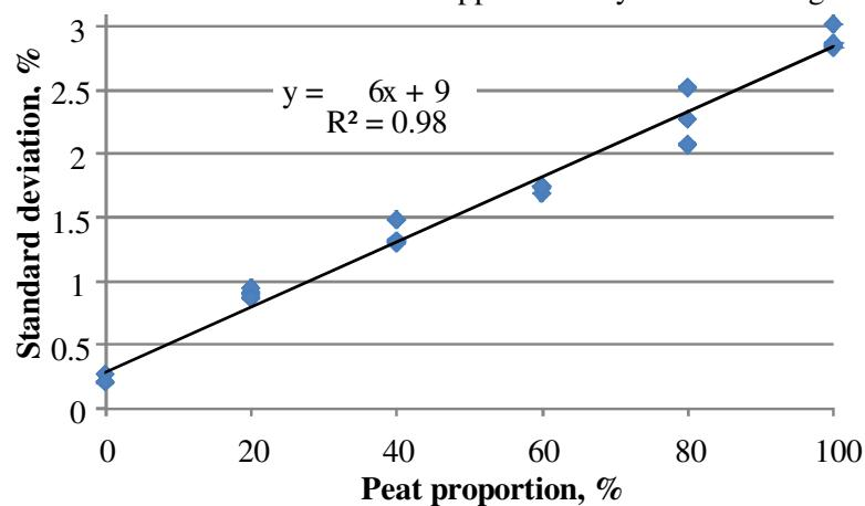
Fig. 7. Standard deviation (pixels) of the distance between straw particles in dependence on peat proportion
