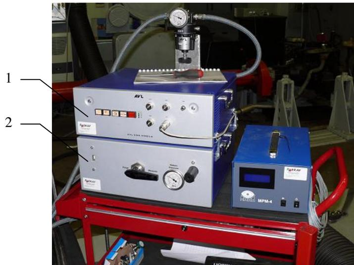
Fig. 2. AVL KMA mobile fuel measuring system: 1 – measuring module; 2 – conditioning module
