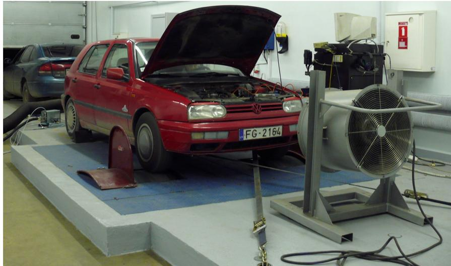
Fig. 3. Laboratory Chassis Dynamometer Mustang MD-1750
