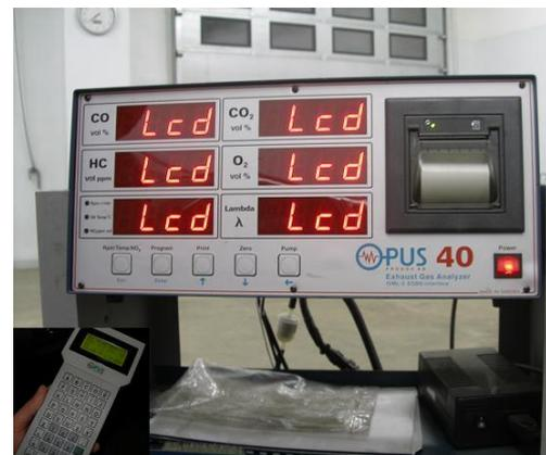
Fig. 6. Gas Analyzer OPUS 40
