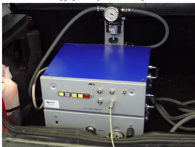
Fig. 5. Fuel consumption meter AVL KMA Mobile
