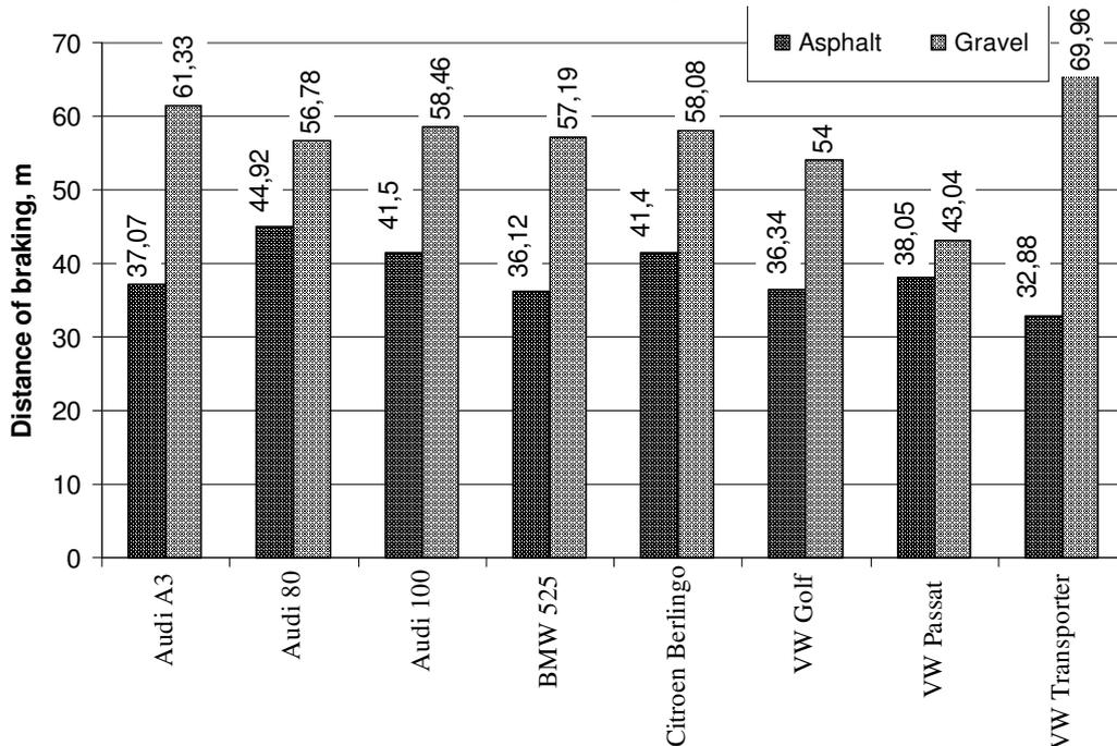
Fig. 3. Distances of braking for test cars on asphalt and gravel roads
