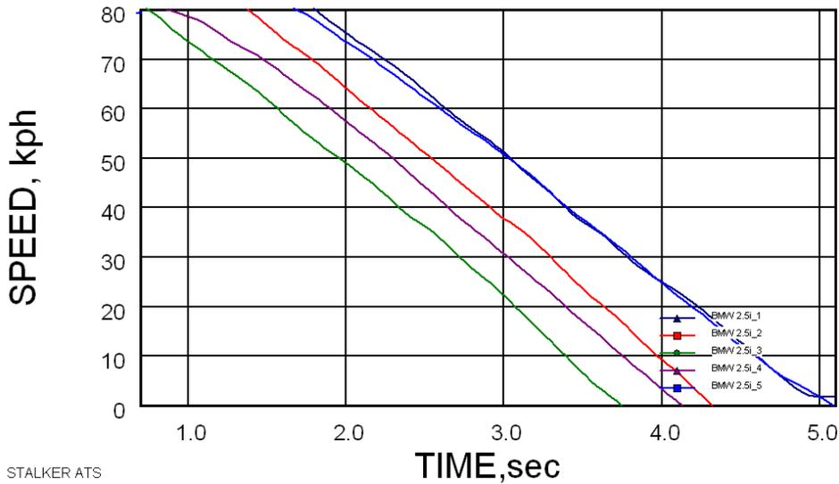
Fig. 2. Period of braking for a car BMW 525, starting braking at 80 km h<sup>-1</sup> (Stalker ATS software window screen shot)
