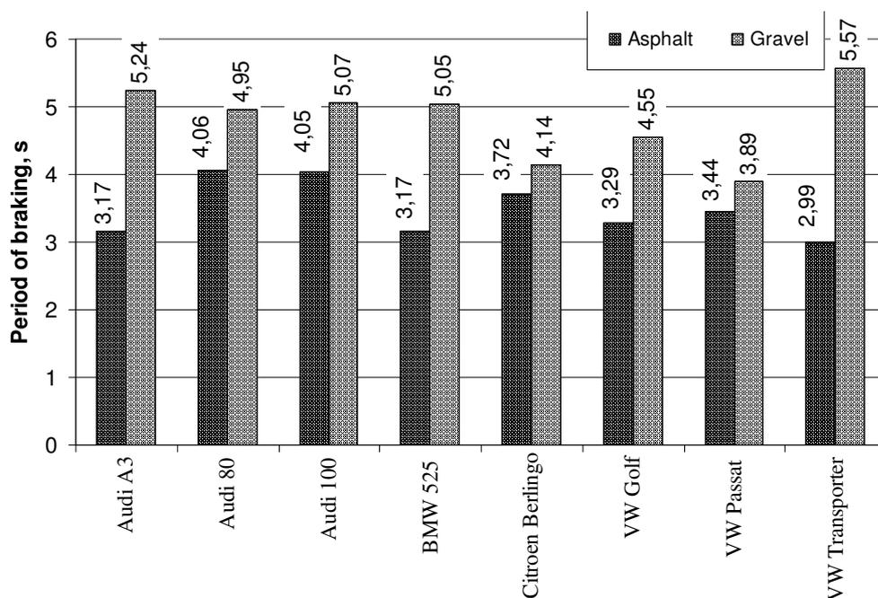
Fig. 4. Periods of braking for cars on asphalt and gravel roads
