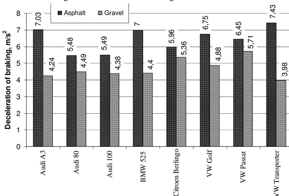
Fig. 5. Comparison of average deceleration rates of braking for cars
