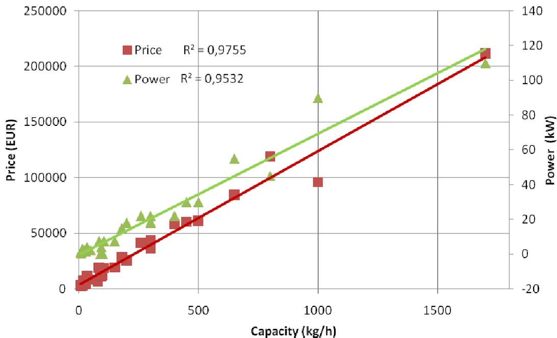
**Fig. 3. Interconnection of oil-pressing equipment power and price considering capacity**
