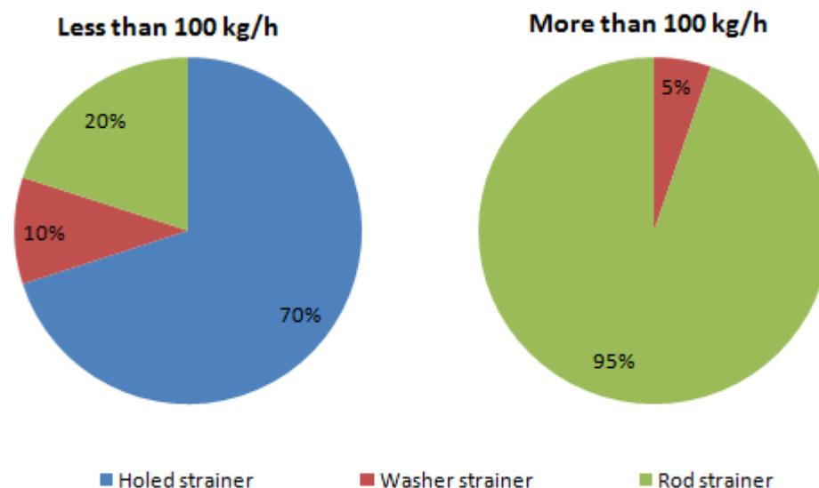
Fig. 7. The percentage of oil-pressing equipment according to strainer constructions
