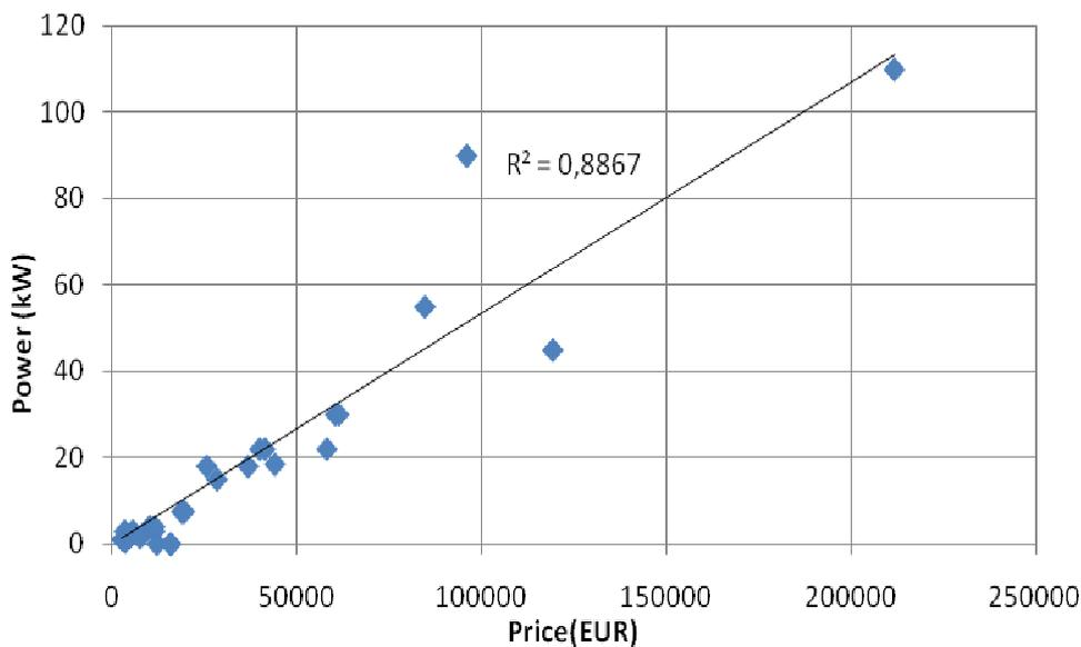
**Fig. 4. Interconnection of oil-pressing equipment power and price**
