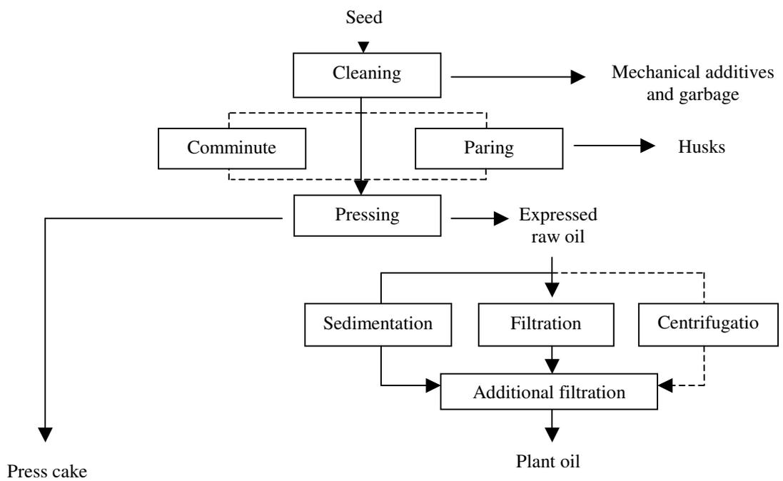
Fig. 2. Processing oil-seed in (local) small devices
