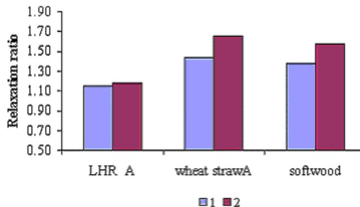
Fig. 1. Relaxation ratios after 2 min (1) and 24 h relaxation (2) for granules by pressing the disperse biofuels at 150 MPa
