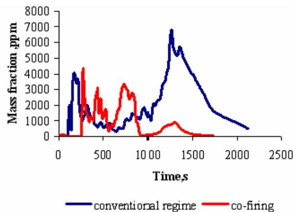
Fig. 3. Time dependence variations of CO emission during the burnout LHR B granules for the self-sustaining and co-firing regimes
