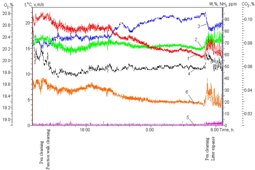
**Fig. 3. Daily change of numeric values of indoor climate parameters in Pigsty C:**
