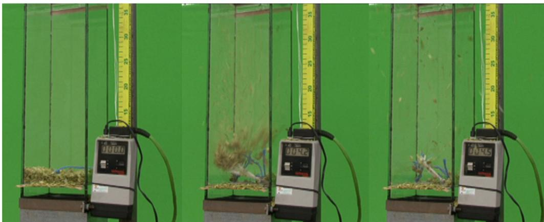
Fig. 7. Behaviour of crushed hops and strings mixture in air-flow
