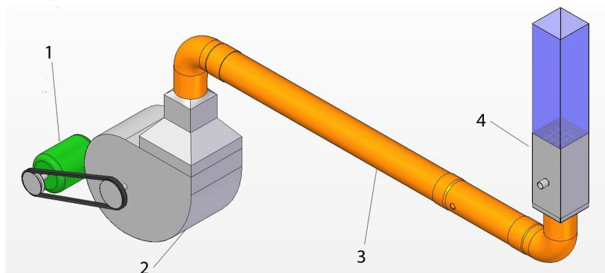
Fig. 5. Diagram of the apparatus used to determine critical speeds in air-flow
