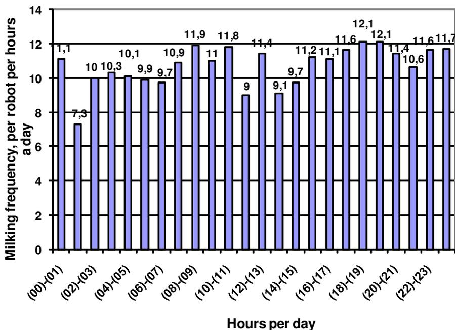
Fig. 3. The total milking capacity per milking robot per hours a day for both robots
