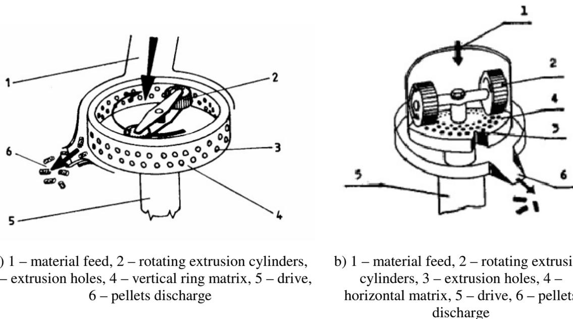
Fig. 2. Operating principle of a braker with vertical matrix (a) and with horizontal matrix (b)
