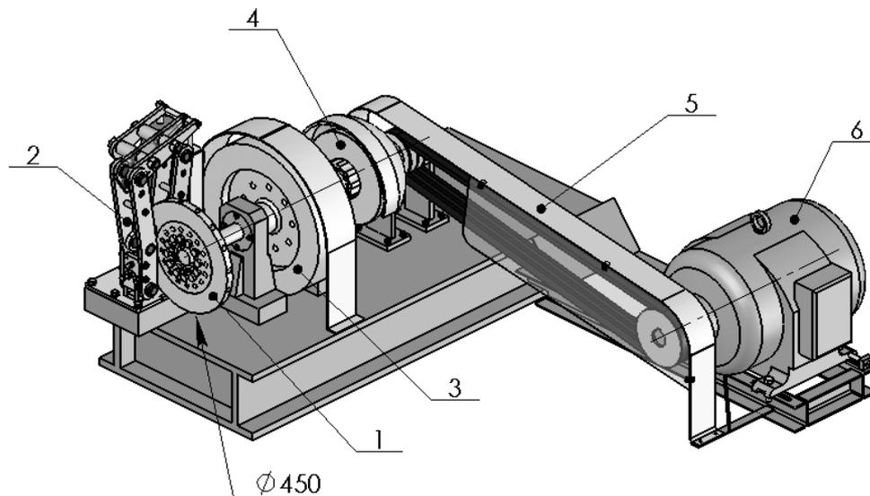
Fig. 1. **Inertia stand:** 1 – disc; 2 – disc brake DBE-1; 3 – flywheel;
