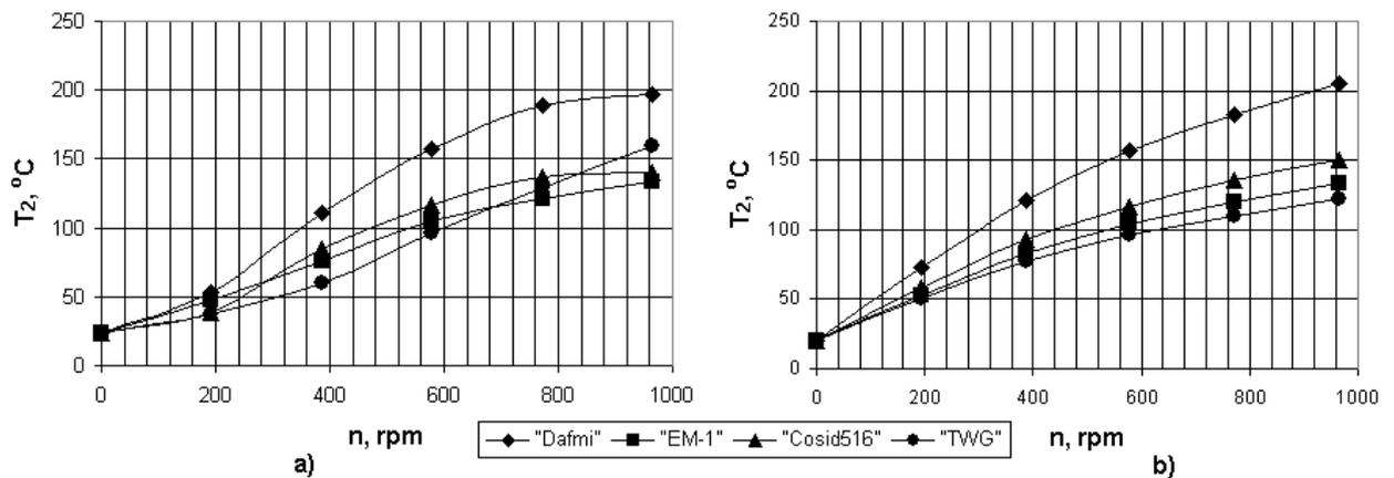
Fig. 2. The friction lining thermal balance temperature  $T_2$  depending on a disc revolutions  $n$  at the beginning of braking ( $p = 1.15$  MPa,  $R = 2$  time/min):
