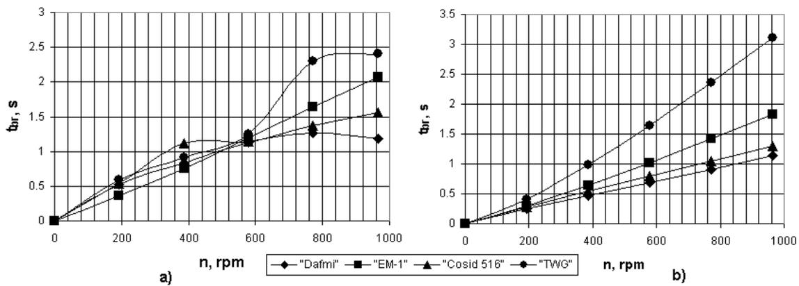
Fig. 4. The braking time  $t_{br}$  depending on a disc revolutions  $n$  at the beginning of braking ( $p = 1.15$  MPa,  $R = 2$  time/min):
