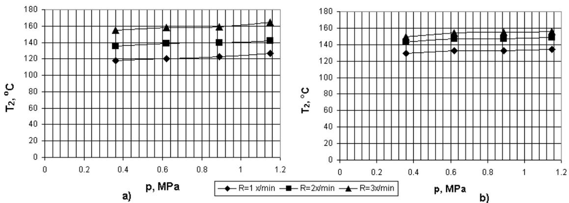
Fig. 5. The friction lining EM-1 thermal balance temperature  $T_2$  depending on specific surface pressure  $p$  and braking intensity  $R$  ( $p = 1.15$  MPa,  $R = 2$  time/min):
