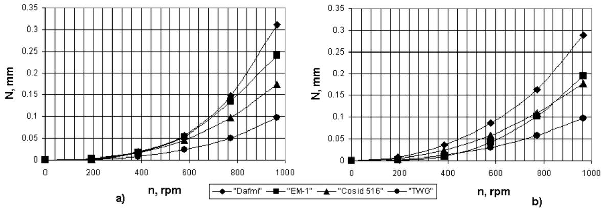
Fig. 3. The wear of friction lining  $N$  depending on a disc revolutions  $n$  at the beginning of braking ( $p = 1.15$  MPa,  $R = 2$  time/min):
