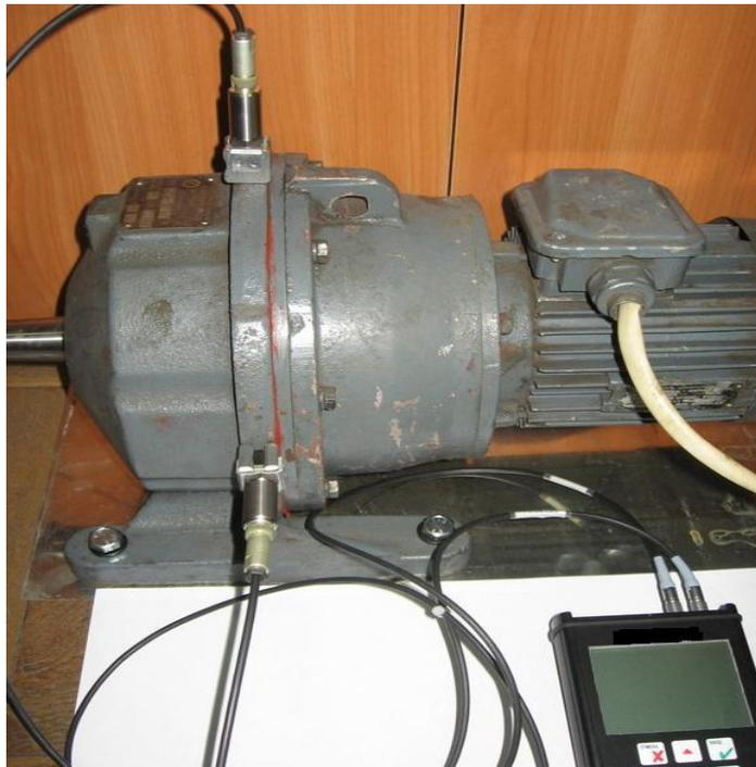
Fig. 1. Planetary reduction gearmotor
