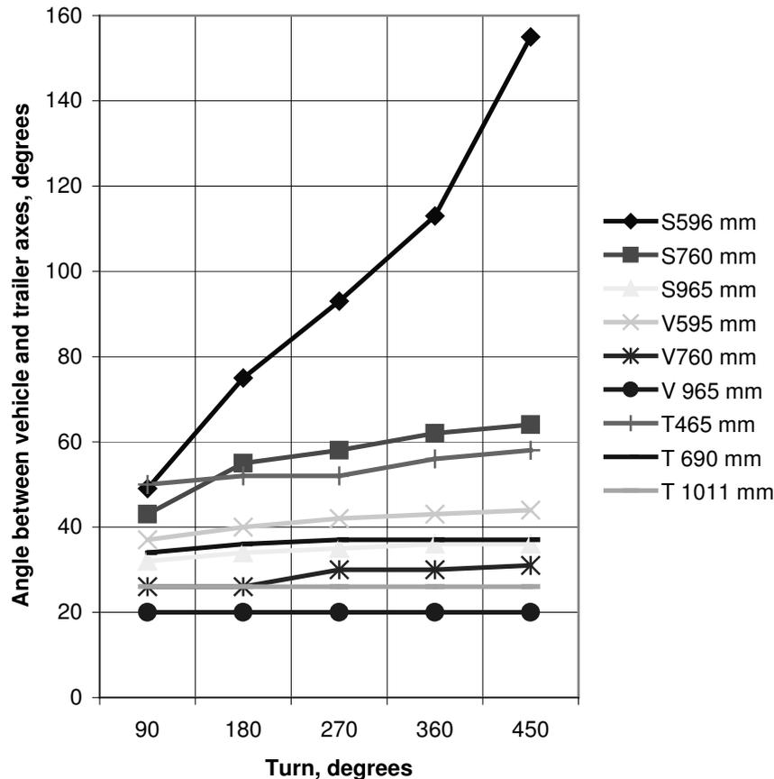
Fig. 4. Angle formed by the axes of the model's semitrailer and towing vehicle
