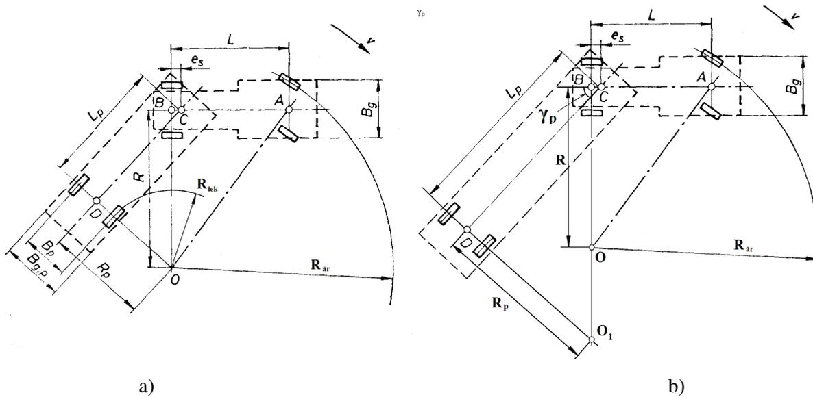
Fig. 2. Kinematics of a road train's turn in movement along a circle
