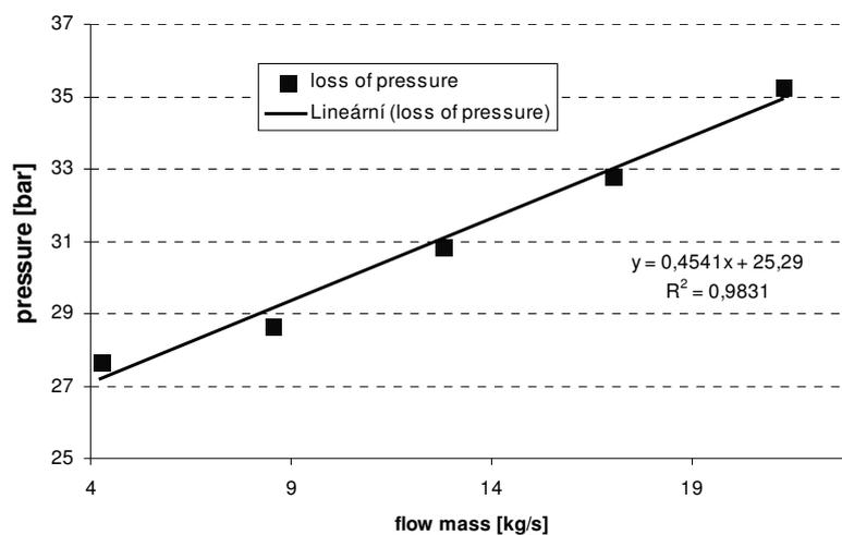
Fig. 3. The loss of pressure on the actuator dependence on the flow mass sugar beets
