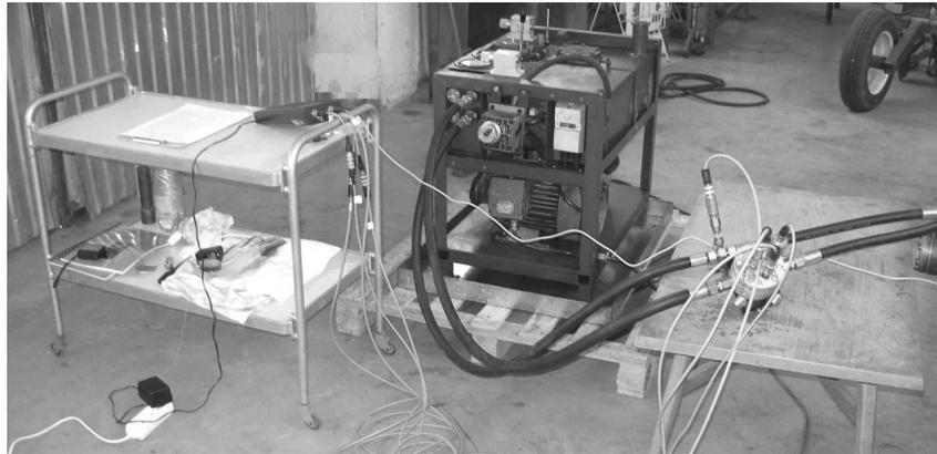
Fig. 1. The configuration for drive the rod sifting conveyor and the measuring apparatus
