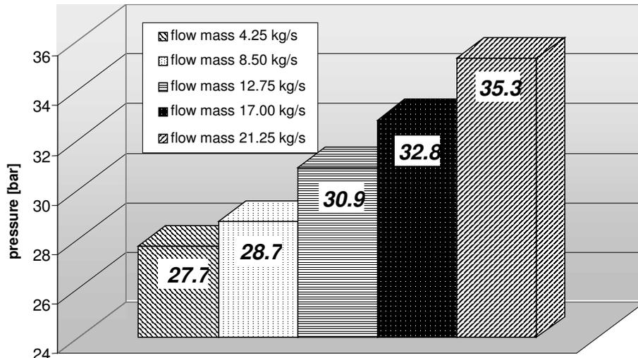
Fig. 4. The loss of pressure on absolute values on the flow mass sugar beets
