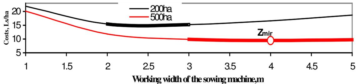
Fig. 2. Changes of variable costs depending on the working width of the sowing machine
