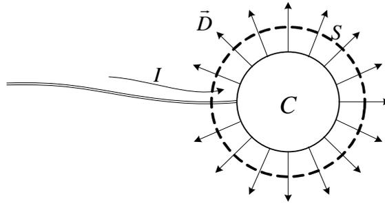
Fig. 6. Full current law in single wire circuit
