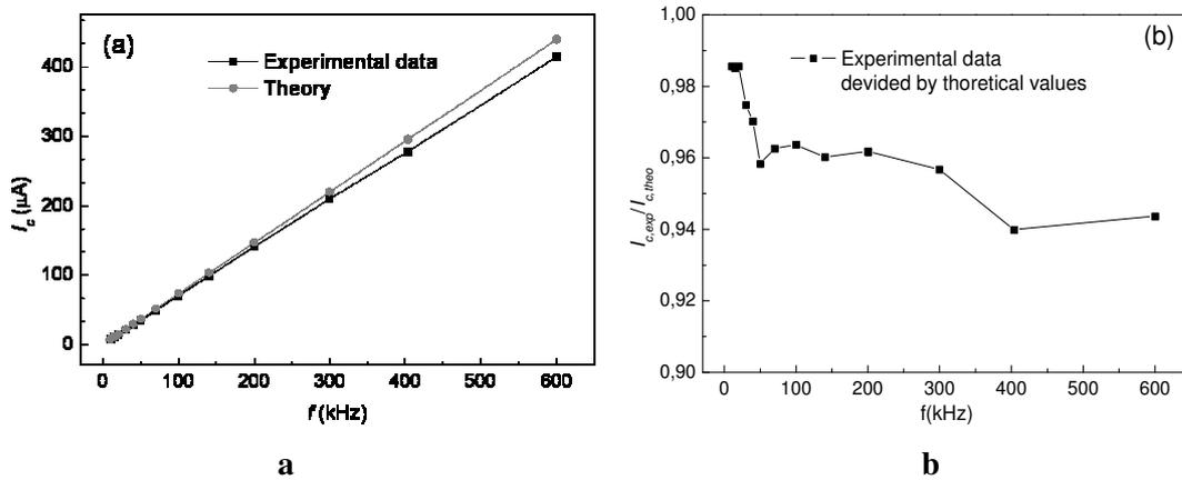
Fig. 2. Measured and theoretical current as a dependence of frequency (2.a) and deviation of measured and theoretical current (2.b) in case of capacity of ball with diameter  $D=20$ mm
