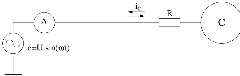
Fig. 1. Single wire line current measuring scheme
