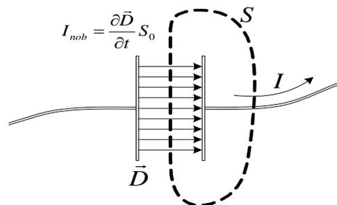
Fig. 5. **Full current law in circuit with ordinary capacitor**
