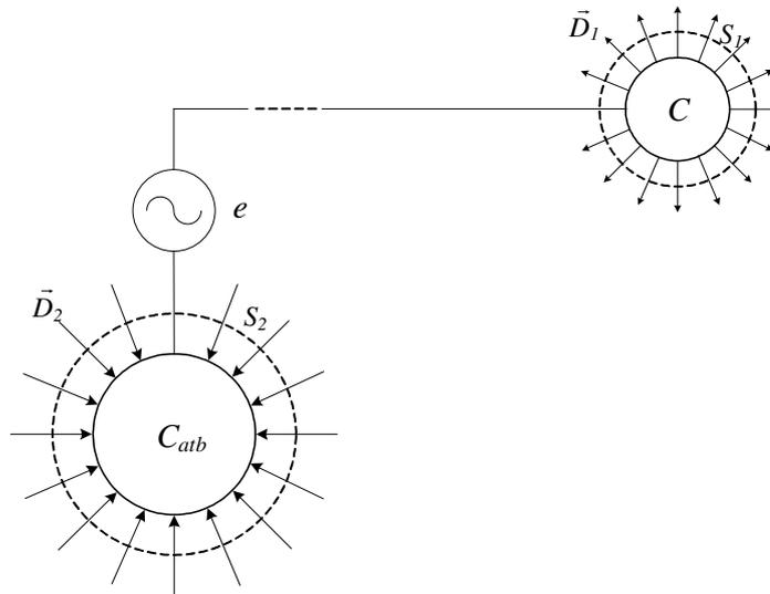
Fig. 7. Single wire scheme with support capacity  $C_{atb}$
