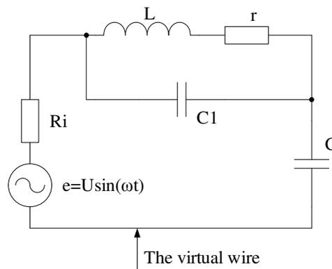
Fig. 4. **The correspondent double wire scheme**
