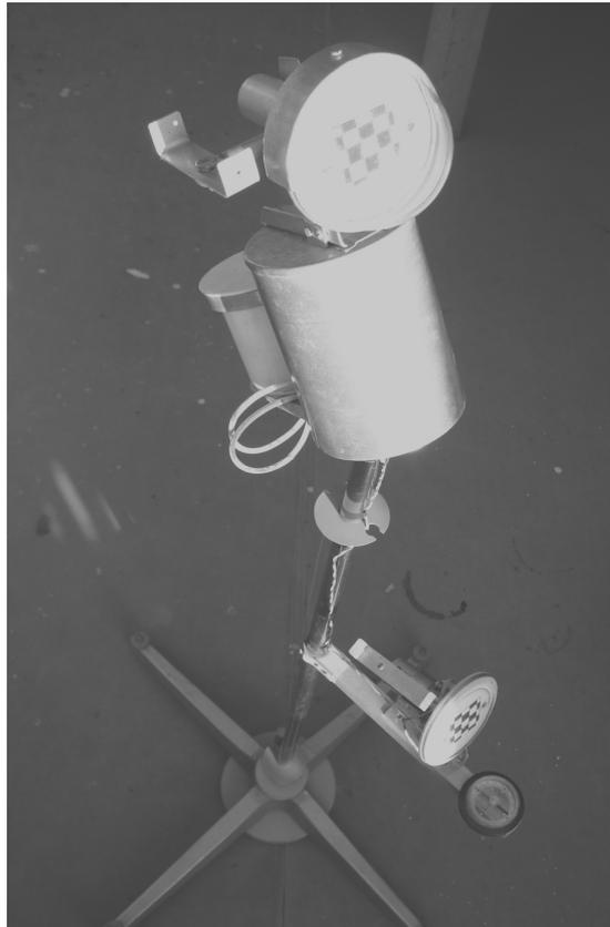
Fig. 1. Device DM-4 for measuring the solar energy
