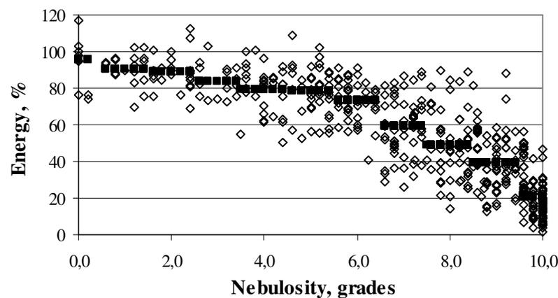
Fig. 5. Dependence of the measured ( $\diamond$ ) and measured mean ( $\blacksquare$ ) daily energy sum received by tracking the sun surface, expressed as percentage from maximal possible one, on the nebulosity
