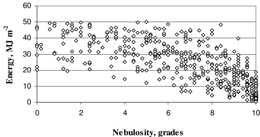
Fig. 4. Dependence of the daily energy sum ( $\text{MJ m}^{-2}$ ) measured with tracking the sun receiver on the nebulosity (grades)
