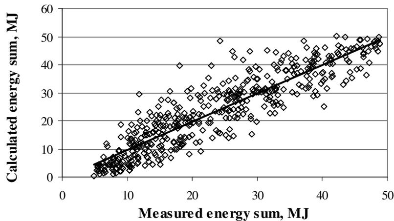
Fig. 8. Comparison of the calculated daily energy sum received by tracking the sun receiver with measured one, both in MJ
