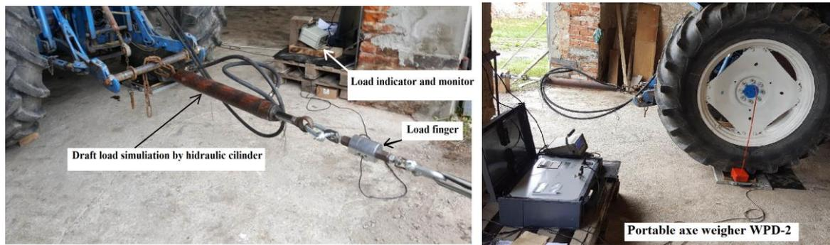
Fig. 2. Measuring of axis weight when draft force was simulated by the hydraulic cylinder
