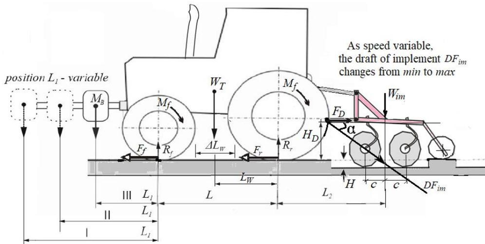
Fig. 3. Scheme of aggregate and acting forces,  $L_2 = 1.8$  m,  $M_B = 120$  kg
