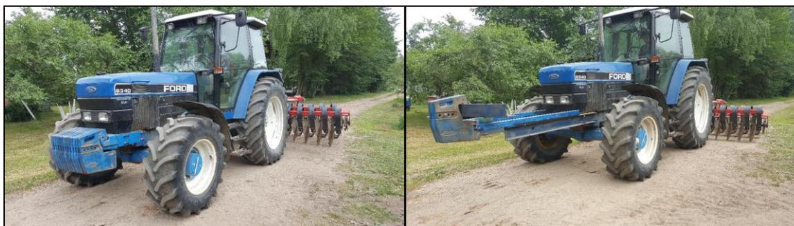
Fig. 1. Front ballast by default (a) and front ballast with a possibility to change its forward distance (b)
