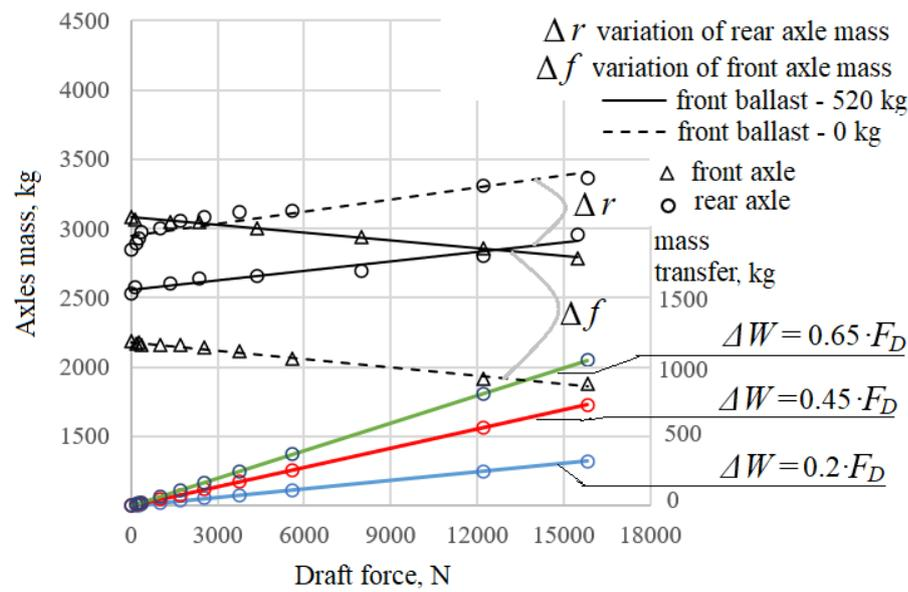
Fig. 4. Variation of front and rear axle weight according to draft force
