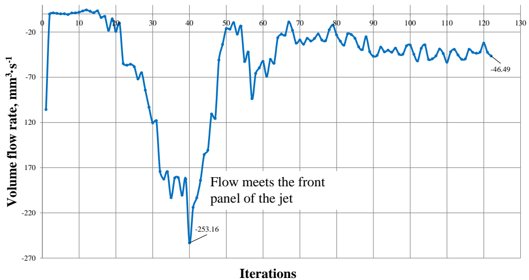
Fig. 4. Volume Flow Rate from SolidWorks Simulation for the original design and stagnation point
