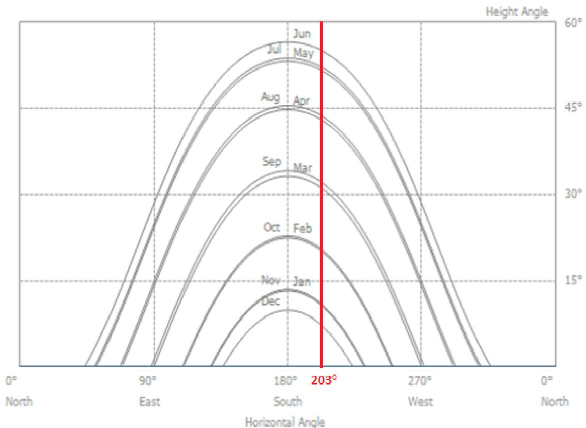
Fig. 1. Solar elevation angle in different months
