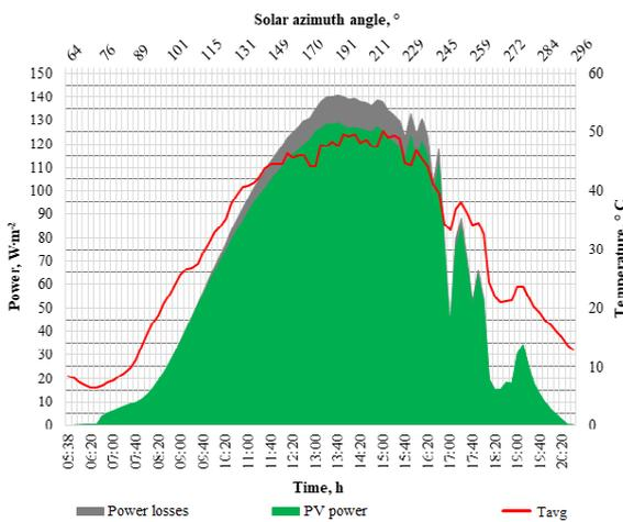
Fig. 12. Solar azimuth angle, PV power and power losses on April 27
