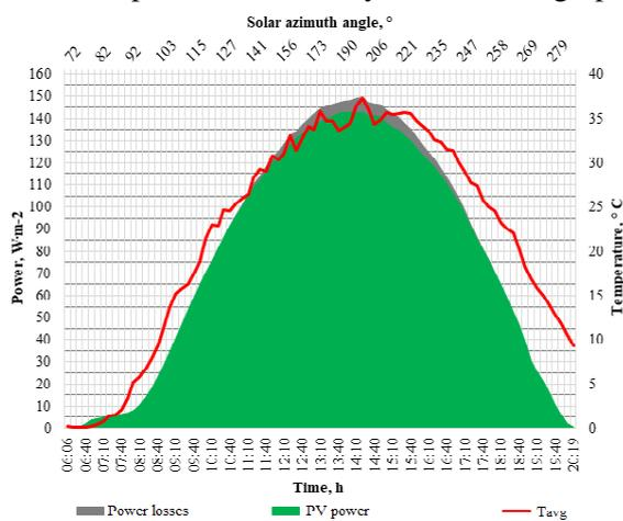
Fig. 10. Solar azimuth angle, PV power and power losses on April 16
