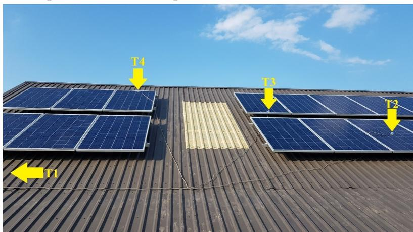
**Fig. 2. Placement of temperature sensors on PV modules:**
