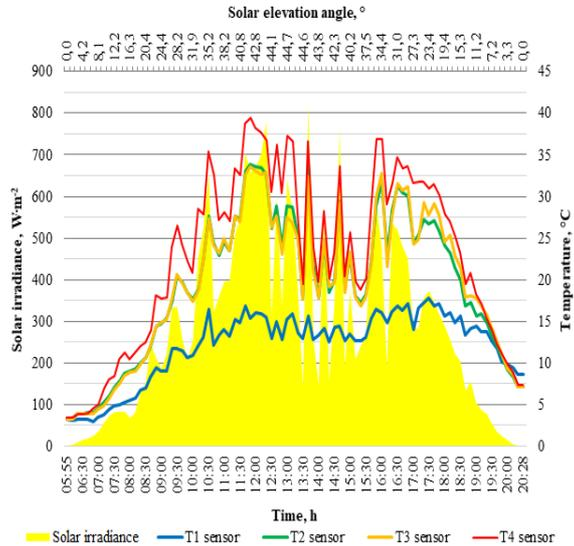
Fig. 7. Solar elevation angle, irradiance and temperature on April 20
