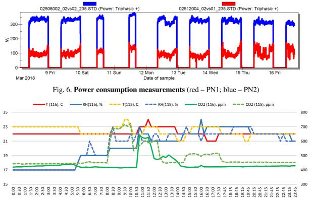
Fig. 7. PN1 and PN2 zone measurement results of LoRaWAN sensors
