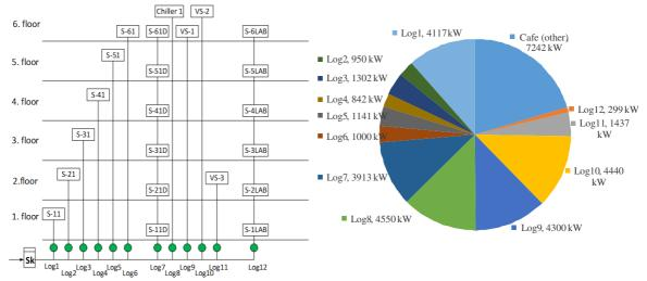
Fig. 2. Schematic diagram of EEF building with distributed area meters (left) and consumed energy distribution diagram by zones (right)
