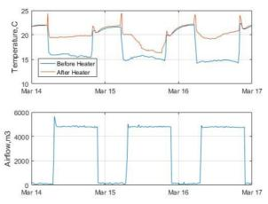
Fig. 5. Experiment results in PN6 zone level using 6 kW heater
