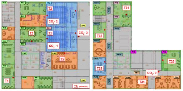
Fig. 1. Faculty building PN zones and sensor placement: first floor (left); sixth floor (right)
