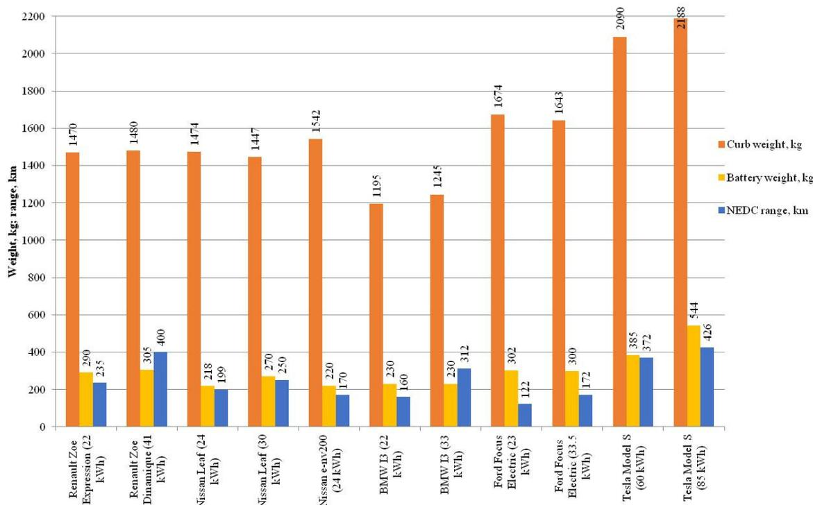
Fig. 3. Battery capacities, gross weights and ranges of electric automobiles according to the NEDC cycle
