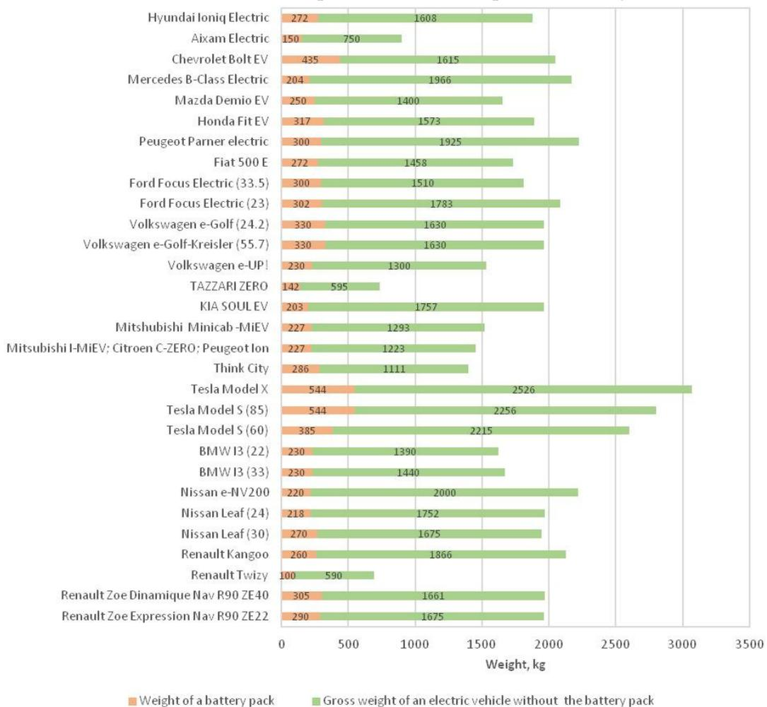
**Fig. 1. Weights of selected electric automobiles and their battery packs**
