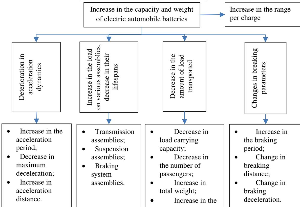
Fig. 2. Effects of the weights of an automobile on its performance parameters
