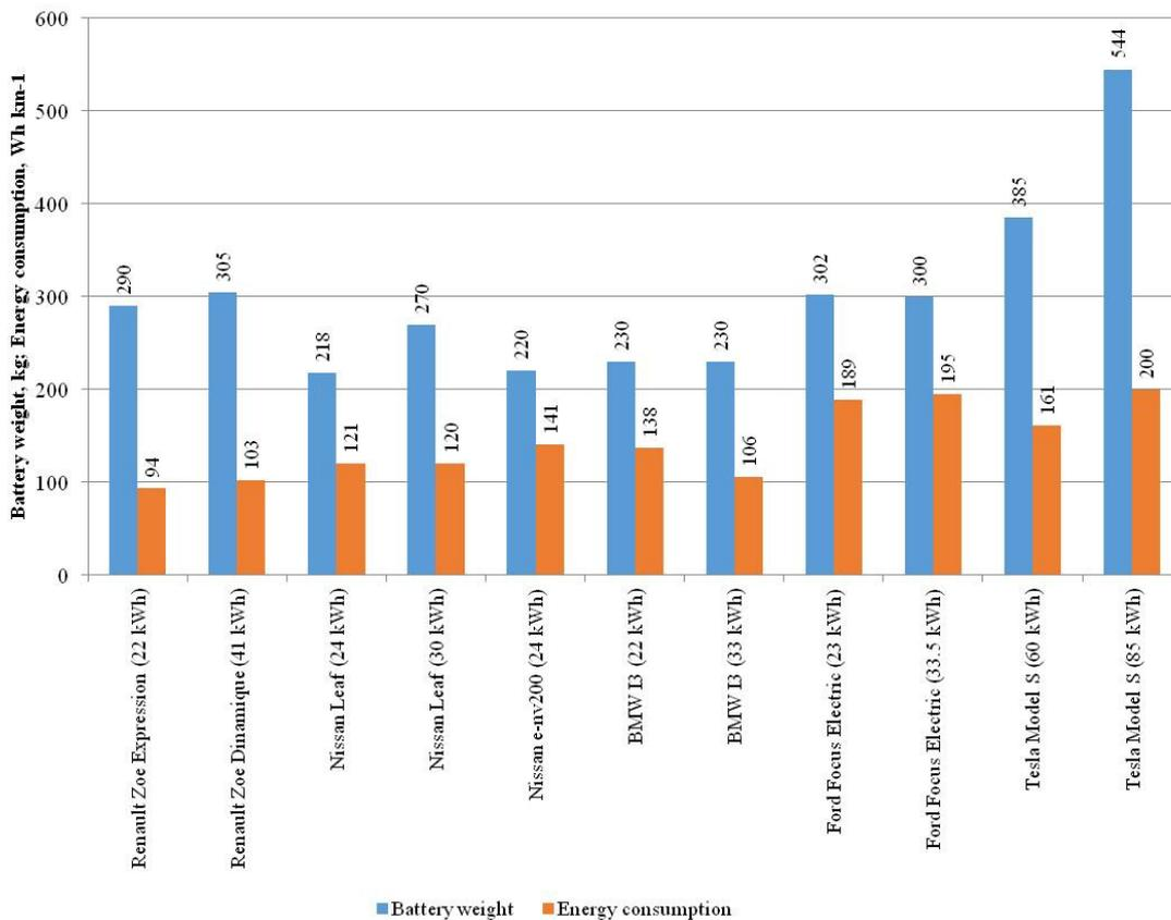
Fig. 4. Battery weights and energy consumption per km travelled for the electric automobiles
