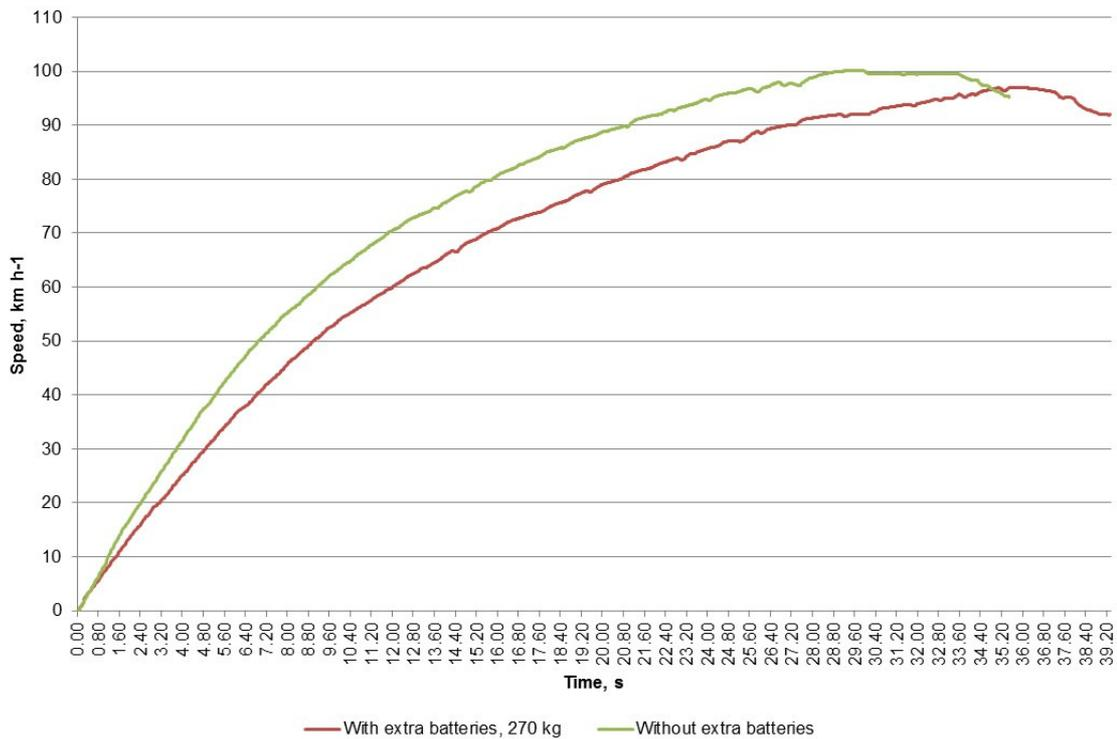
Fig. 5. Change in the acceleration speed of the electric automobile Fiat FiorinoElectrico
