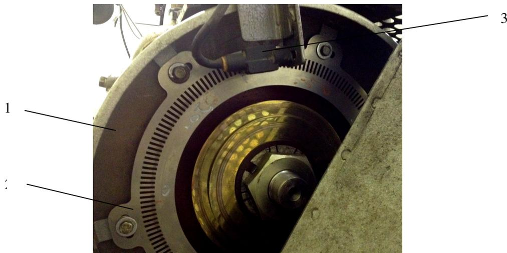
Fig. 2. **Crankshaft encoder:** 1 – flywheel; 2 – encoder target; 3 – VR sensor
