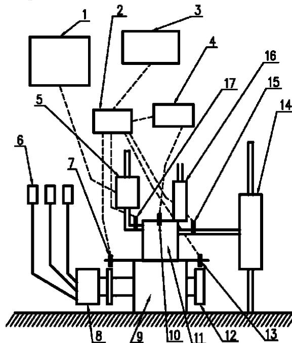
Fig. 1. **IDT-69 engine setup:** 1 – engine control module; 2 – NI 9068 chassis; 3 – host PC; 4 – charge amplifier Kistler 5018A; 5 – inlet air heater; 6 – fuel reservoirs; 7 – camshaft phase HE sensor; 8 – high pressure fuel pump; 9 – cylinder block; 10 – pressure sensor Kistler 6061B; 11 – cylinder head; 12 – flywheel; 13 – flywheel rotation sensor; 14 – exhaust surge tank; 15 – exhaust temperature sensor; 16 – cooling system condenser; 17 – inlet air temperature sensor
