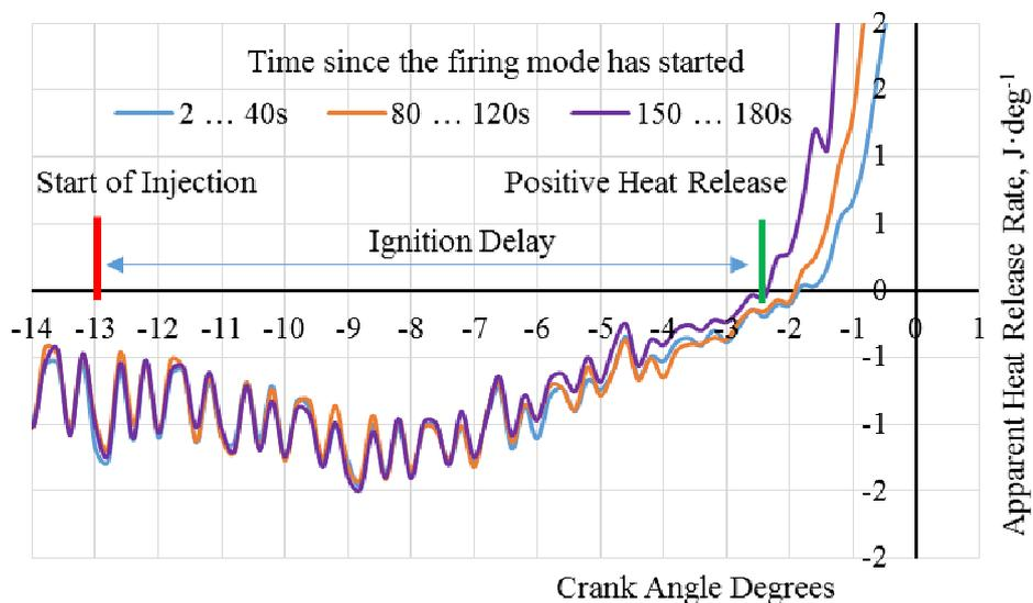
Fig. 4. Assessment of apparent heat release rate
