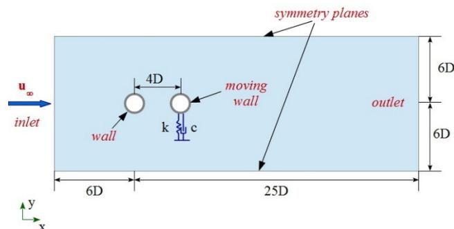
Fig. 3. **Computational domain and boundary conditions of FSI test case:**  $D$  is the diameter of the cylinder,  $k$  is the spring stiffness coefficient,  $c$  is the damping coefficient and  $u_\infty$  is the free-stream velocity
