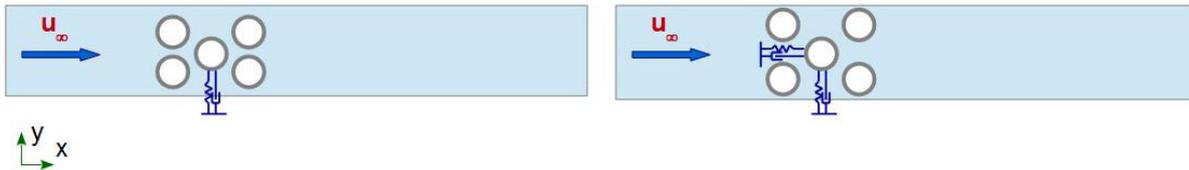
Fig. 4. **Computational domain and dimensions:** left – 1DOF model; right – 2DOF model
