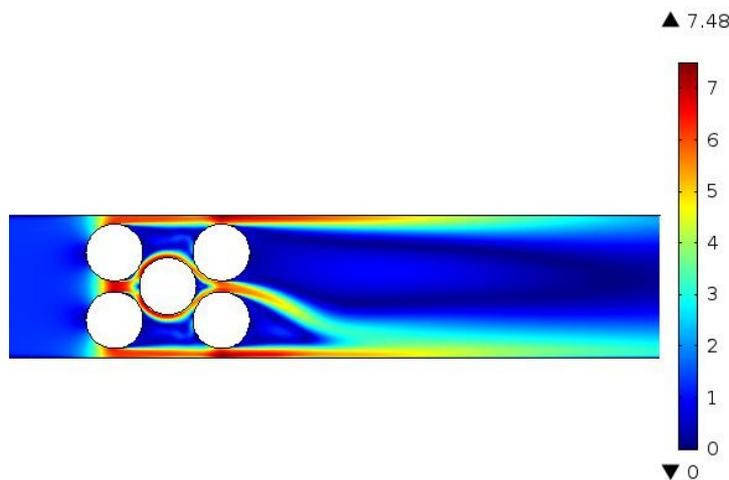
Fig. 5. **Distribution of the velocity magnitude ( $\text{m}\cdot\text{s}^{-1}$ ) around the rod bundle of 1DOF case**
