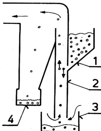
Fig. 2. **Vertical channel (detailed view):** 1 – tray; 2 – vertical (aspiration) channel; 3 – stack; 4 – tray (particles of lower critical speed are carried into this tank)
