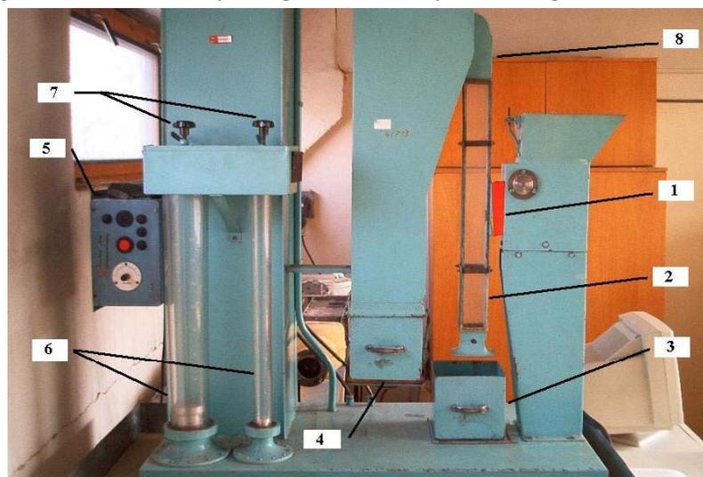
Fig. 1. **Laboratory Air sorter K-293:** 1 – adjustable damper hoppers; 2 – vertical (aspiration) channel; 3, 4 – tanks; 5 – control panel with buttons; 6 – small and large graduated cylinder; 7 – cylinder adjusting screws; 8 – fan
