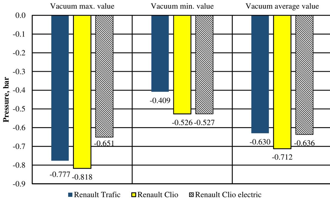
Fig. 5. Changes in the vacuum pressure range for the experimental vehicles
