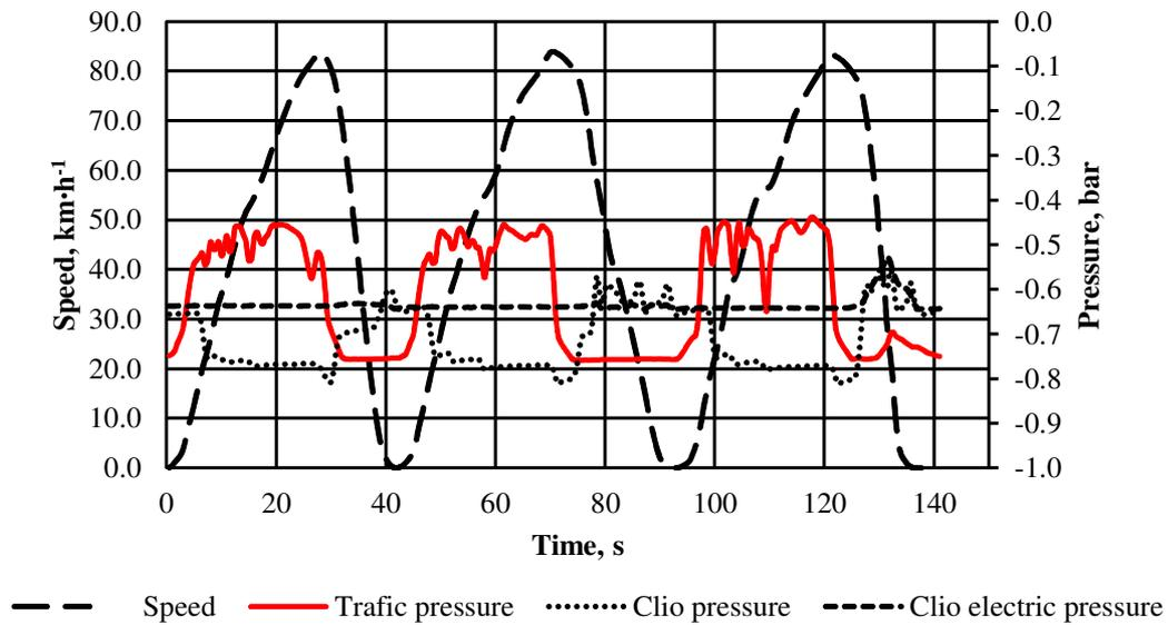
Fig. 4. Changes in the brake booster vacuum pressure depending on the automobile speed and braking regime
