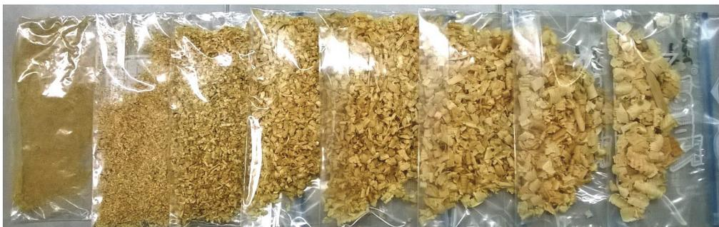
Fig. 6. **Particle size distribution of pine sawdust:** particles retained on the sieve with the largest aperture are on the right, with the smallest aperture are on the left side
