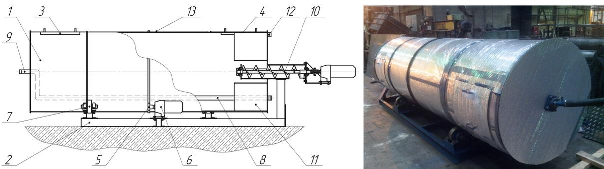
**Fig. 3. Breadboard model of an experimental biofermentation installation of the drum type:** 1 – rotating cylindrical drum; 2 – frame; 3 – charge hole; 4 – checking hole; 5 – power unit; 6 – motor reduction unit; 7 – mounting assemble; 8 – aeration pipe; 9 – air duct for outside air supply; 10 – discharging auger conveyor; 11 – blades; 12 – exhaust duct; 13 – heat insulation
