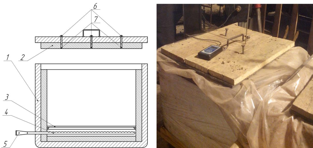
**Fig. 2. Breadboard model of an experimental biofermentation installation of the chamber type:** 1 – biofermentor chamber; 2 – removable lid; 3 – perforated plate; 4 – perforated zigzag pipe; 5 – air compressor nozzle; 6 – plugs; 7 – holes for temperature and oxygen content measurements
