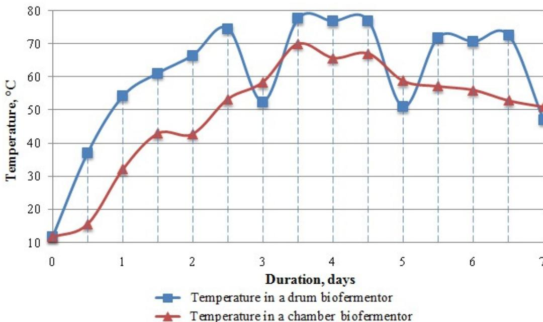
Fig. 5. Graph of the temperature pattern during biofermentation in the chamber and drum type installations
