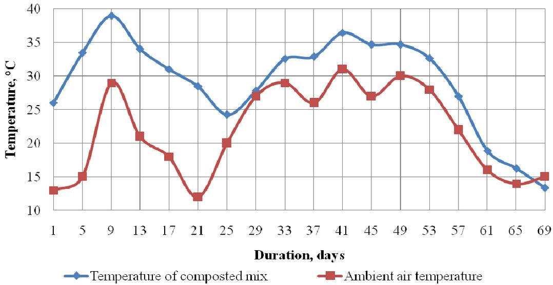
Fig. 4. Graph of the temperature dynamics pattern under the passive pile composting
