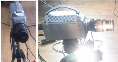
Fig. 3. Phantom V 10.0 Camera
