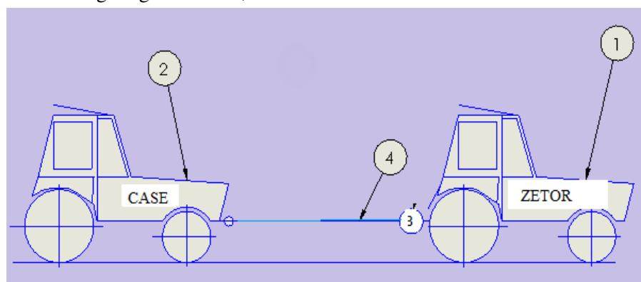
Fig. 1. Research scheme: 1 – tractor Case IH Farmall U Pro 115; 2 – tractor Zetor 10540; 3 – pulling force measurement device; 4 – rigid connection
