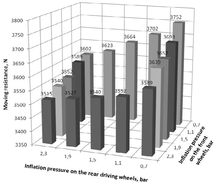
Fig. 3. Tractor 4x2 moving resistance force dependences on different inflation pressure on the front and rear tires on hard surface road
